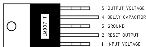
Figure 2. Order Number LM9071T/Flow LB03 See NS Package Number T05D
