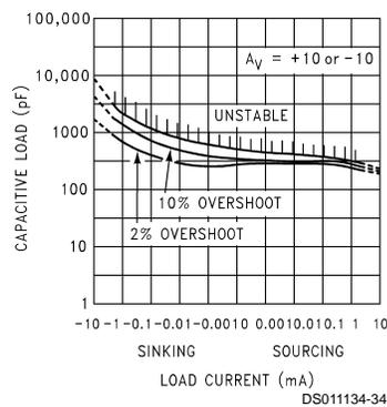
**Note:** Avoid resistive loads of less than 500Ω, as they may cause instability.
