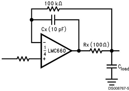
**FIGURE 3. Rx, Cx Improve Capacitive Load Tolerance**
