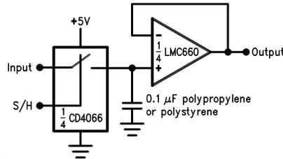
Figure 14. Low-Leakage Sample-and-Hold
