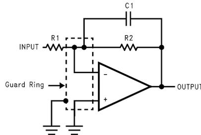
Figure 8. (a) Inverting Amplifier
