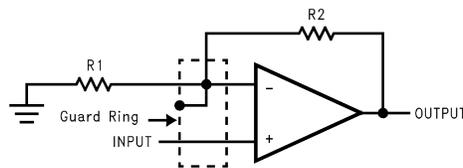
Figure 9. (b) Non-Inverting Amplifier
