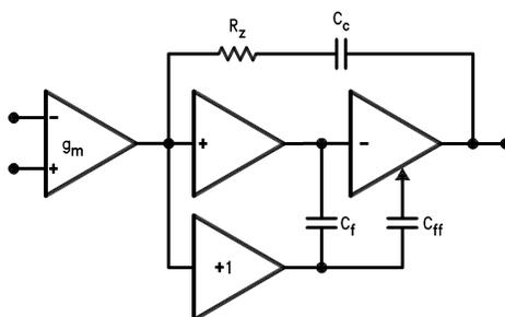
Figure 3. LMC660EP Circuit Topology (Each Amplifier)
