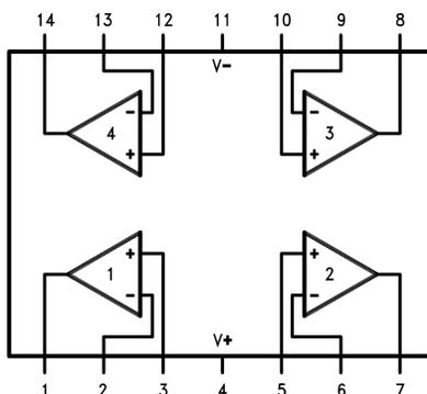
Figure 1. 14-Pin DIP/SO
