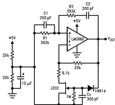
Figure 16. Sine-Wave Oscillator
