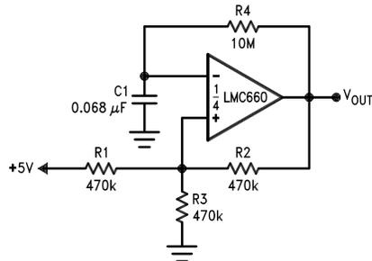
**Figure 17. 1 Hz Square-Wave Oscillator**
