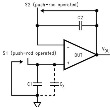
**Figure 13. Simple Input Bias Current Test Circuit**
