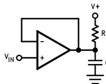
**Figure 6. Compensating for Large Capacitive Loads with a Pull Up Resistor**
