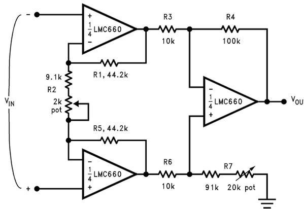
Figure 15. Instrumentation Amplifier
