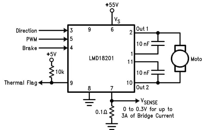
**Figure 15. Current Sensing**
