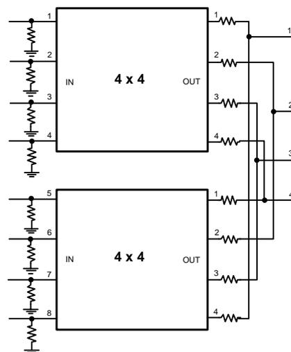
Figure 35. Input Expansion with Separate Termination Resistors
