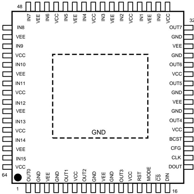
Figure 1. 64-Pin Exposed Pad HTQFP
