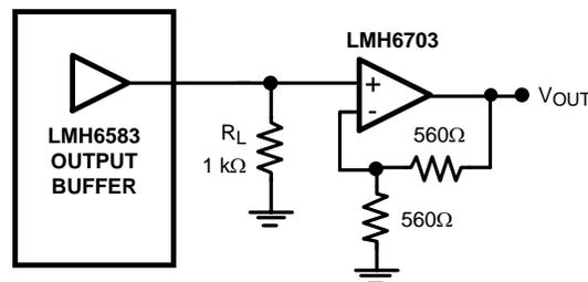
Figure 38. Buffered Output
