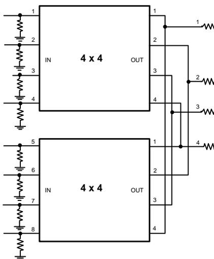
Figure 34. Input Expansion with Shared Termination Resistors
