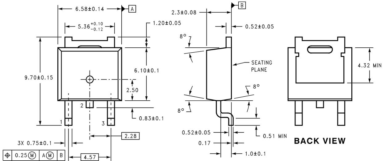
**DIMENSIONS ARE IN MILLIMETERS**
