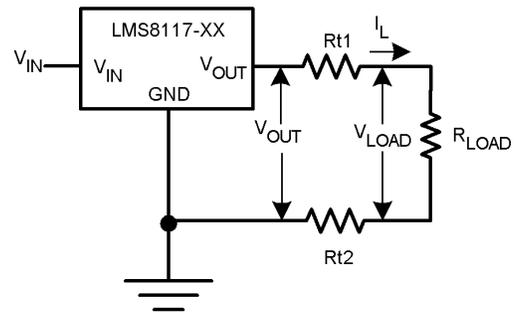
$$V_{LOAD} = V_{OUT} - I_L (Rt1 + Rt2)$$
