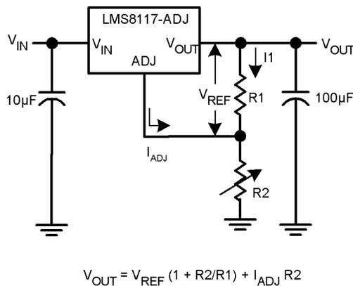
$$V_{OUT} = V_{REF} (1 + R2/R1) + I_{ADJ} R2$$
