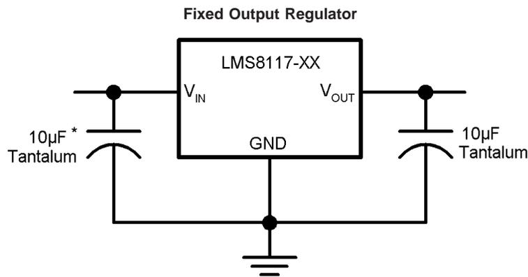
\*Required if the regulator is located far from the power supply filter
