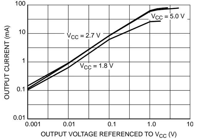
Figure 3. Sourcing Current vs. Output Voltage ( $T_A = 25^\circ\text{C}$ )
