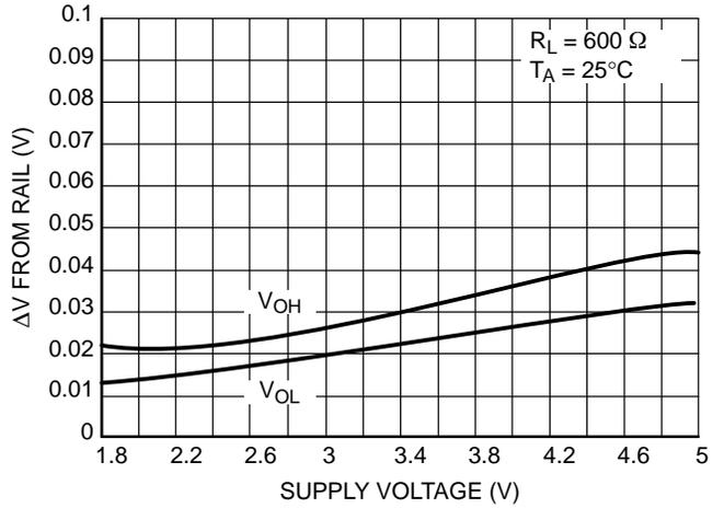
Figure 5. Output Voltage Swing vs. Supply Voltage
