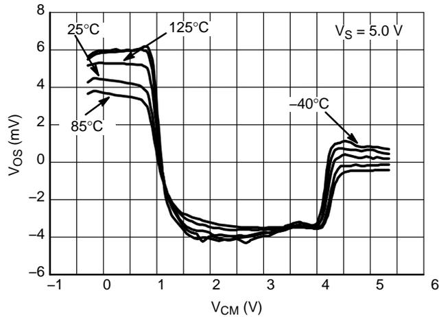
**Figure 26. Offset Voltage vs. Common Mode Range  $V_{DD} 5.0\text{ V}$**
