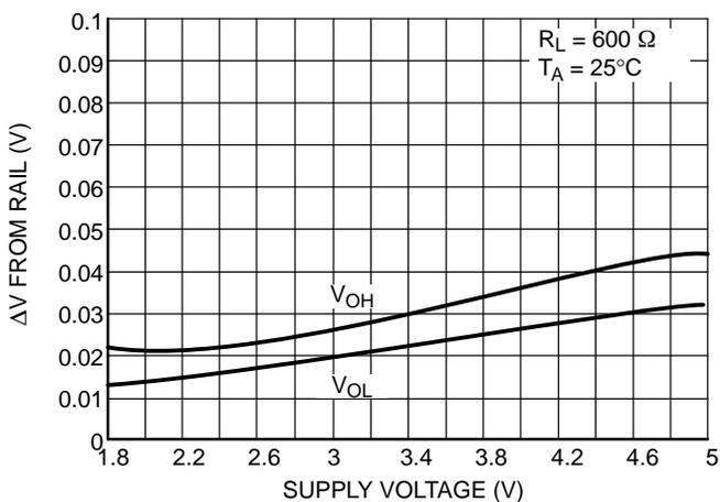
Figure 1. Output Voltage Swing vs. Supply Voltage
