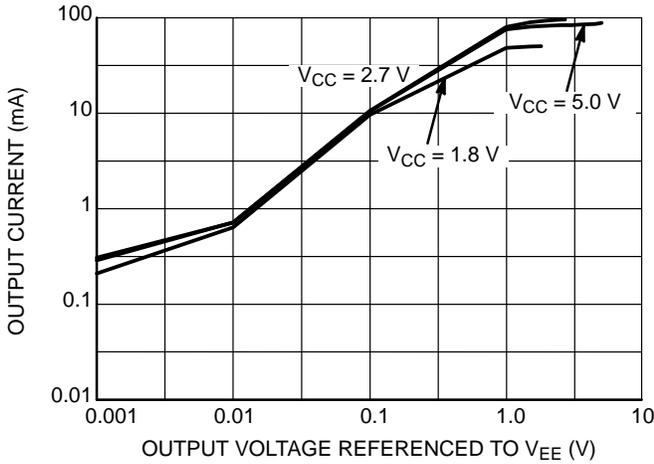
Figure 4. Sinking Current vs. Output Voltage ( $T_A = 25^\circ\text{C}$ )
