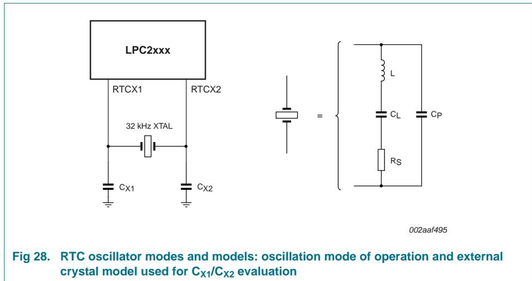
**Fig 28. RTC oscillator modes and models: oscillation mode of operation and external crystal model used for  $C_{X1}/C_{X2}$  evaluation**
