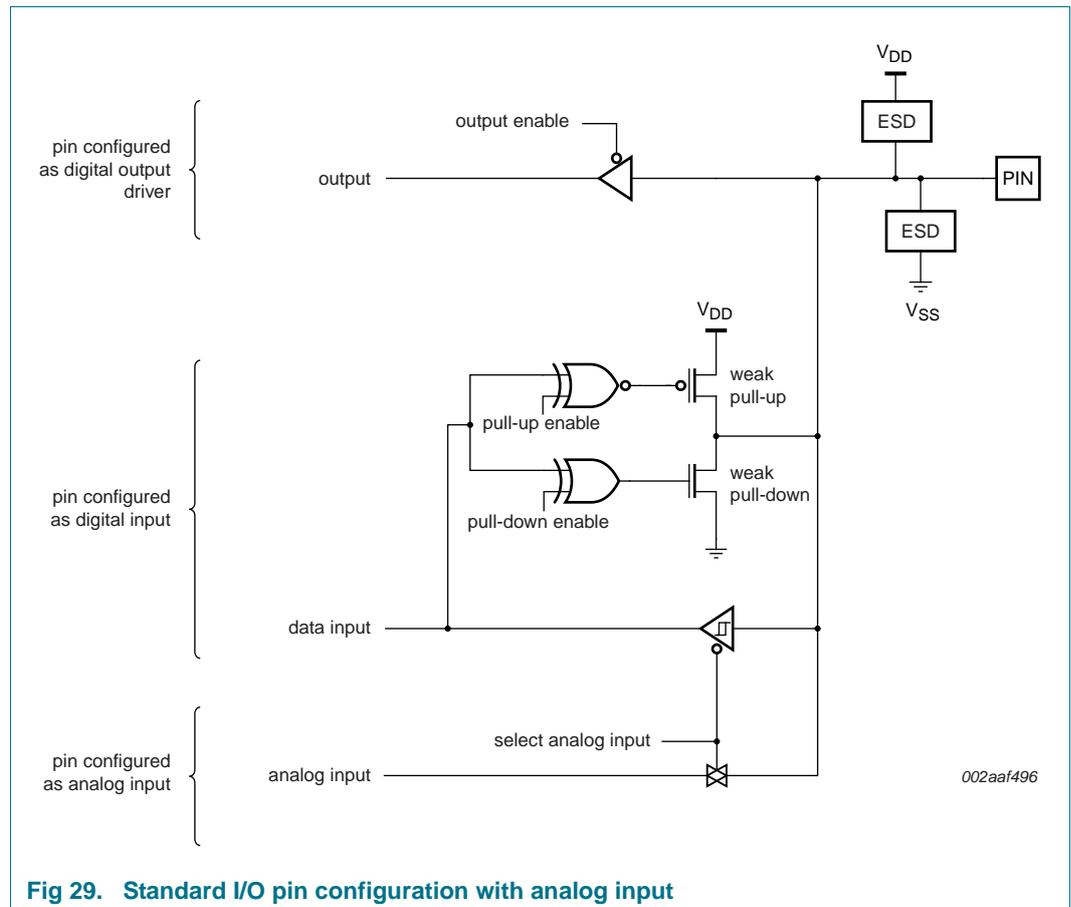
Fig 29. Standard I/O pin configuration with analog input
