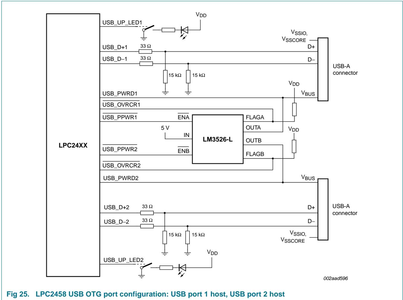
Fig 25. LPC2458 USB OTG port configuration: USB port 1 host, USB port 2 host
