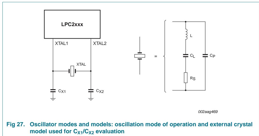
Fig 27. Oscillator modes and models: oscillation mode of operation and external crystal model used for  $C_{X1}/C_{X2}$  evaluation
