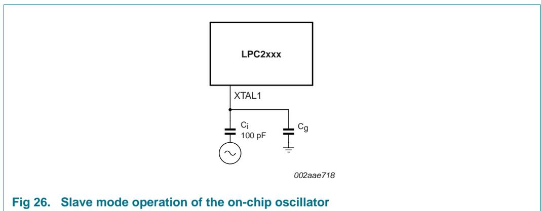
Fig 26. Slave mode operation of the on-chip oscillator
