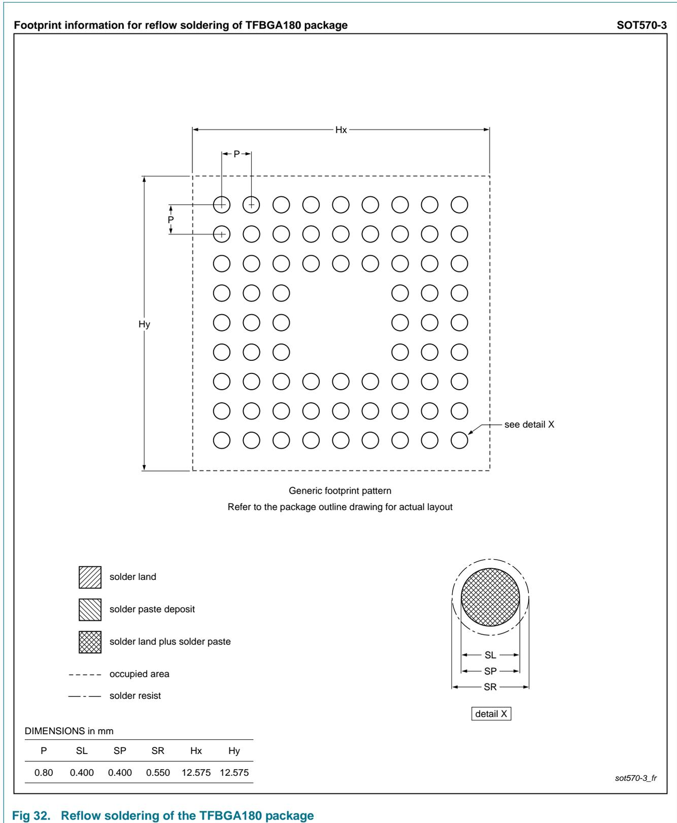
**Fig 32. Reflow soldering of the TFBGA180 package**
