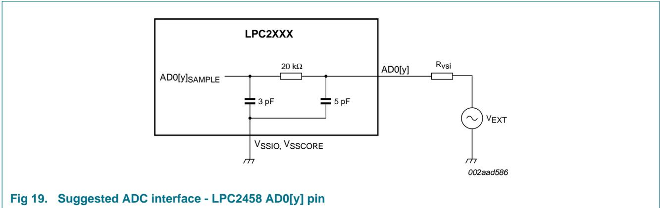
Fig 19. Suggested ADC interface - LPC2458 AD0[y] pin
