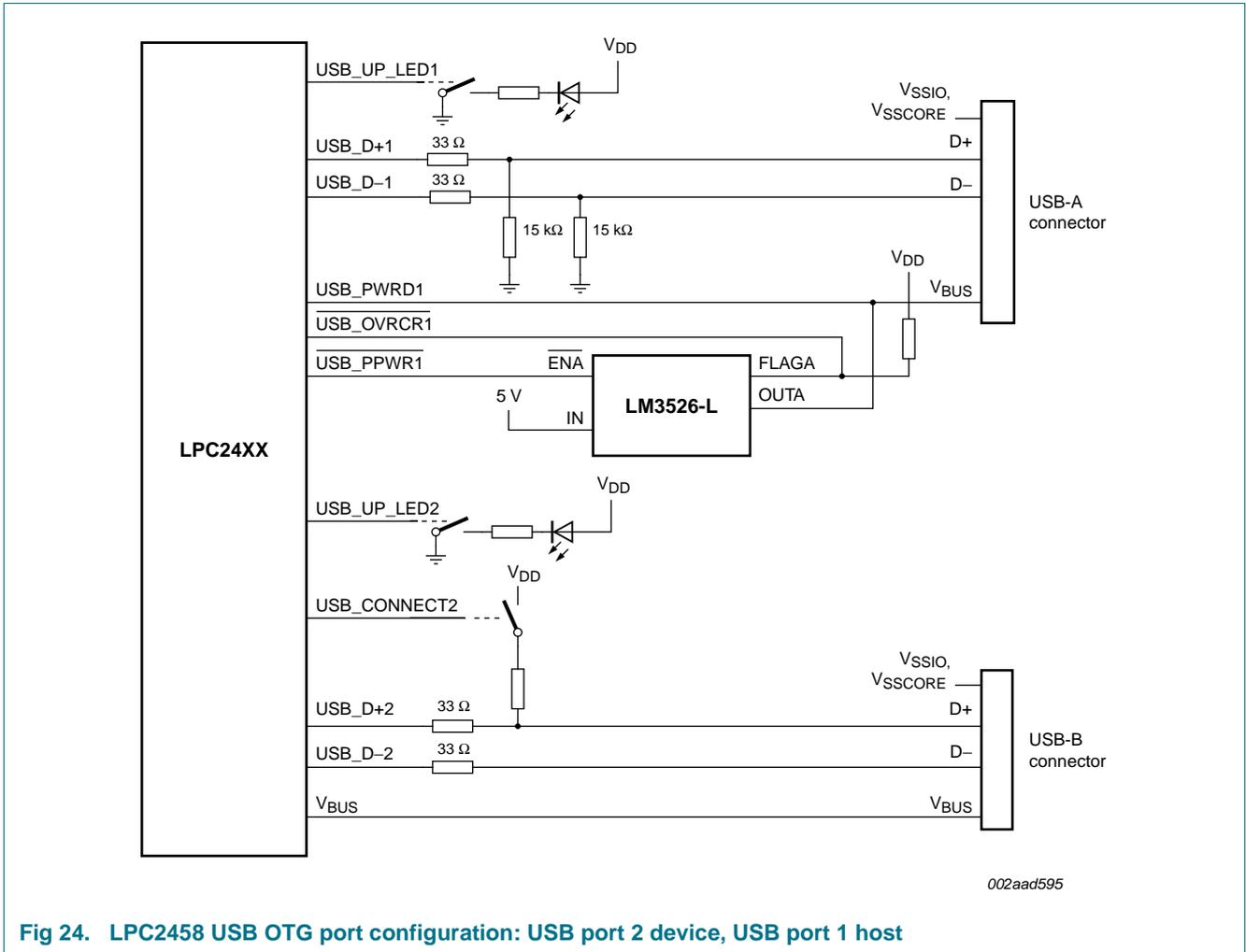
Fig 24. LPC2458 USB OTG port configuration: USB port 2 device, USB port 1 host
