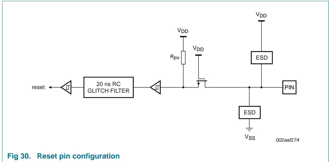
Fig 30. Reset pin configuration
