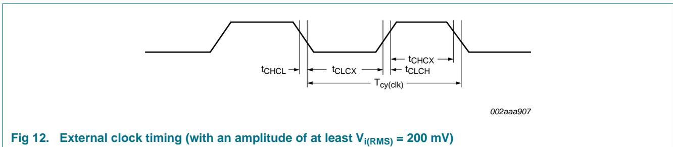
**Fig 12. External clock timing (with an amplitude of at least  $V_{i(RMS)} = 200\text{ mV}$ )**
