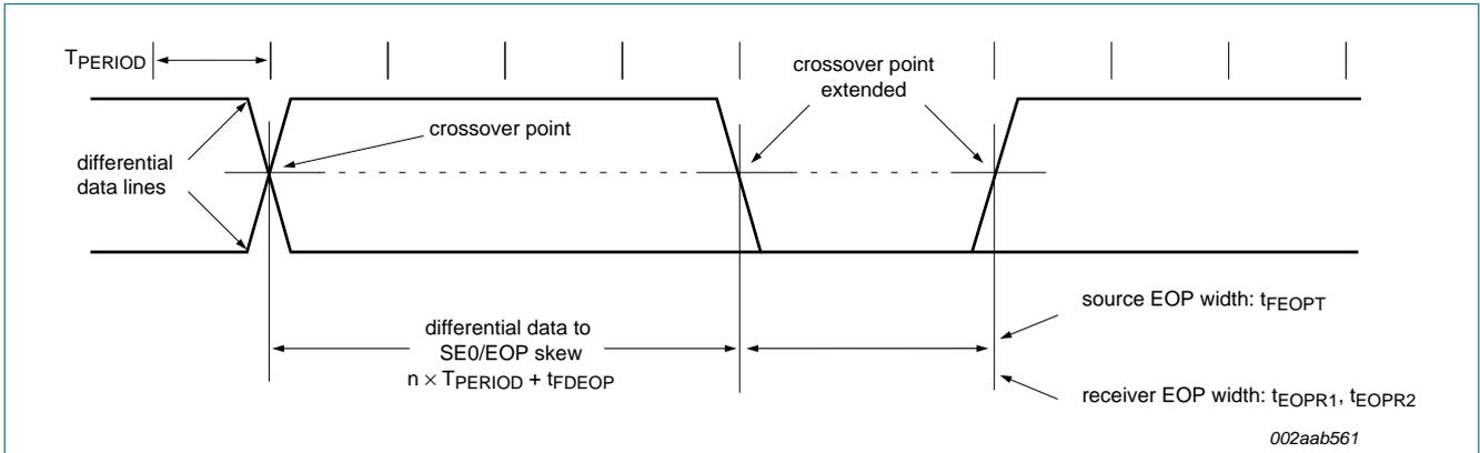
Fig 15. Differential data-to-EOP transition skew and EOP width
