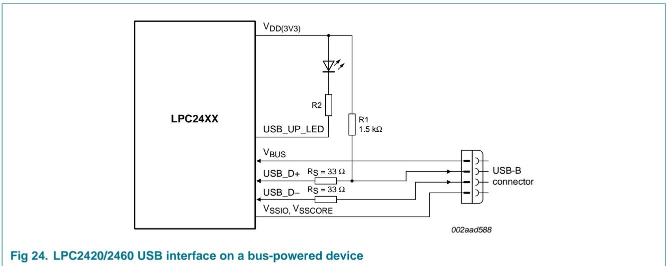
Fig 24. LPC2420/2460 USB interface on a bus-powered device
