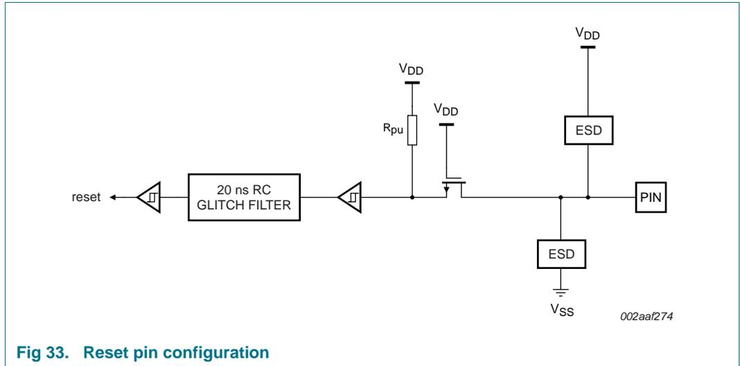
Fig 33. Reset pin configuration
