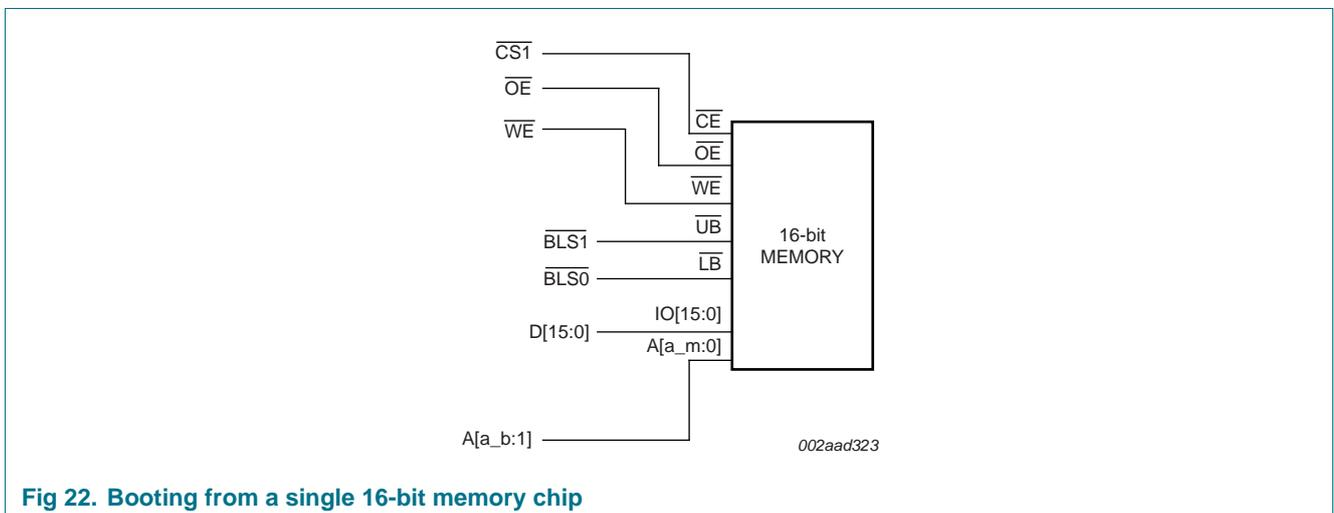
**Fig 22. Booting from a single 16-bit memory chip**
