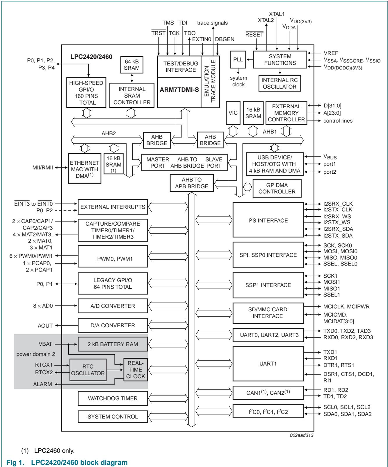
Fig 1. LPC2420/2460 block diagram
