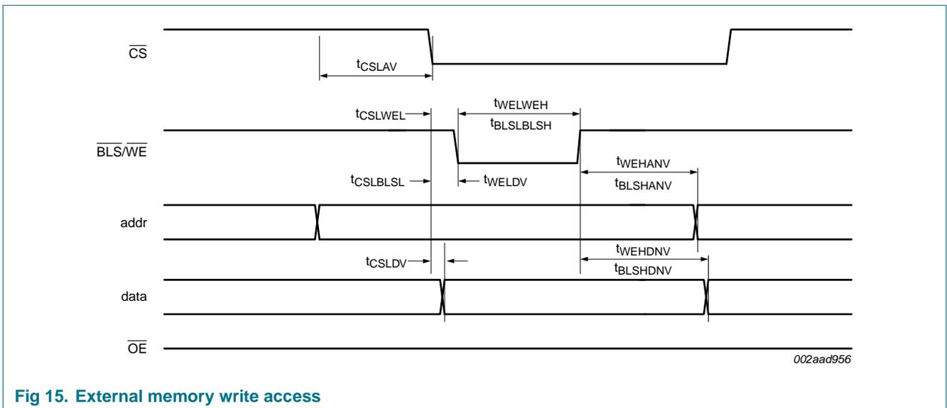
Fig 15. External memory write access
