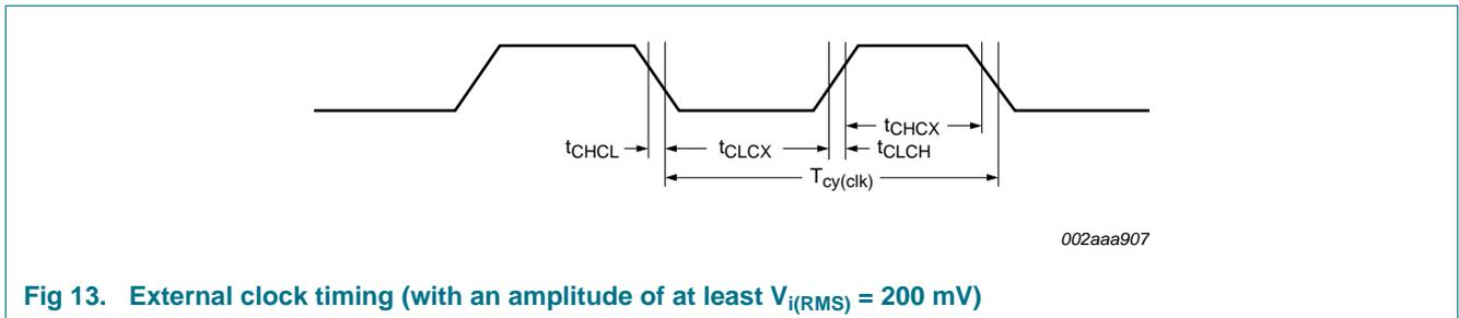
**Fig 13. External clock timing (with an amplitude of at least  $V_{i(RMS)} = 200\text{ mV}$ )**
