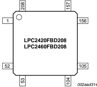
Fig 2. LPC2420/2460 pinning LQFP208 package
