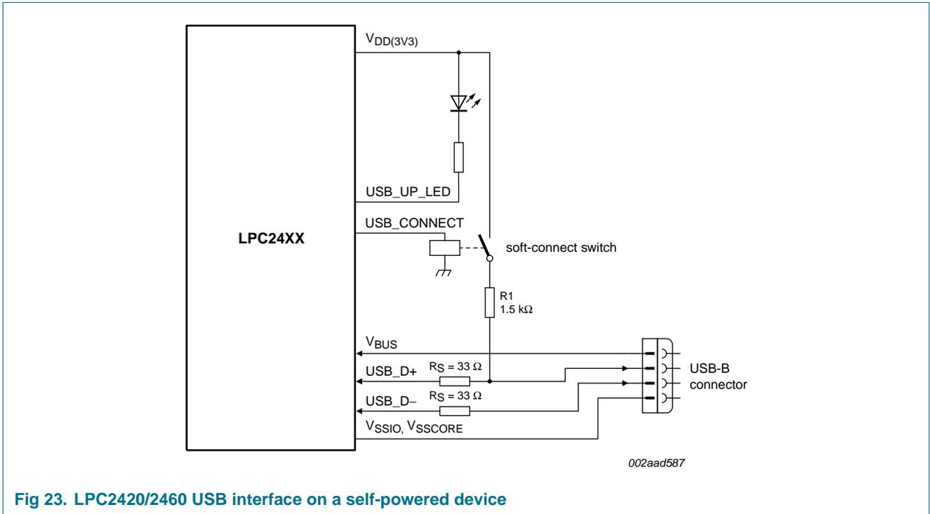
Fig 23. LPC2420/2460 USB interface on a self-powered device
