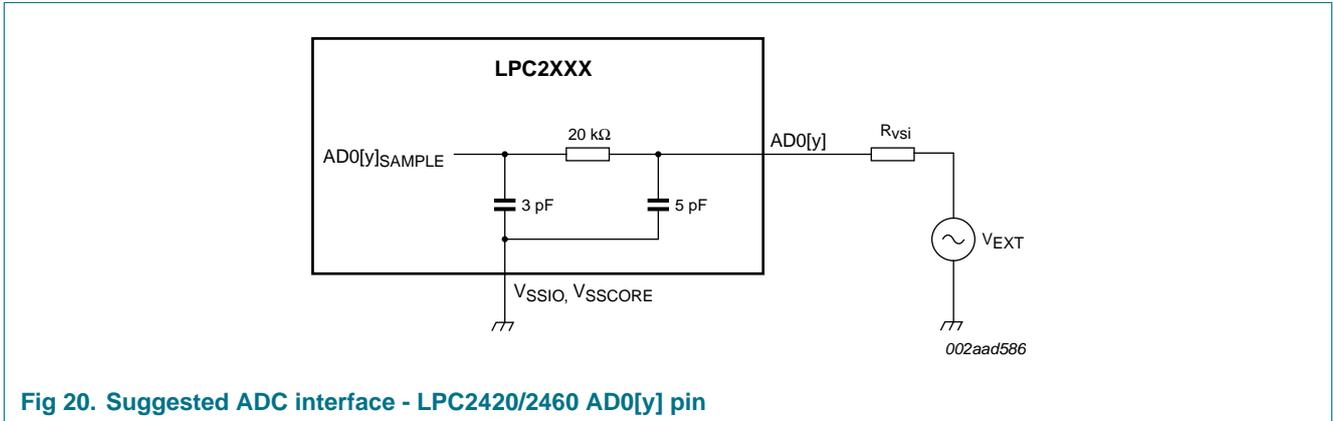
Fig 20. Suggested ADC interface - LPC2420/2460 AD0[y] pin
