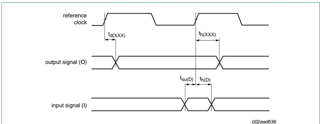
Fig 18. Signal timing
