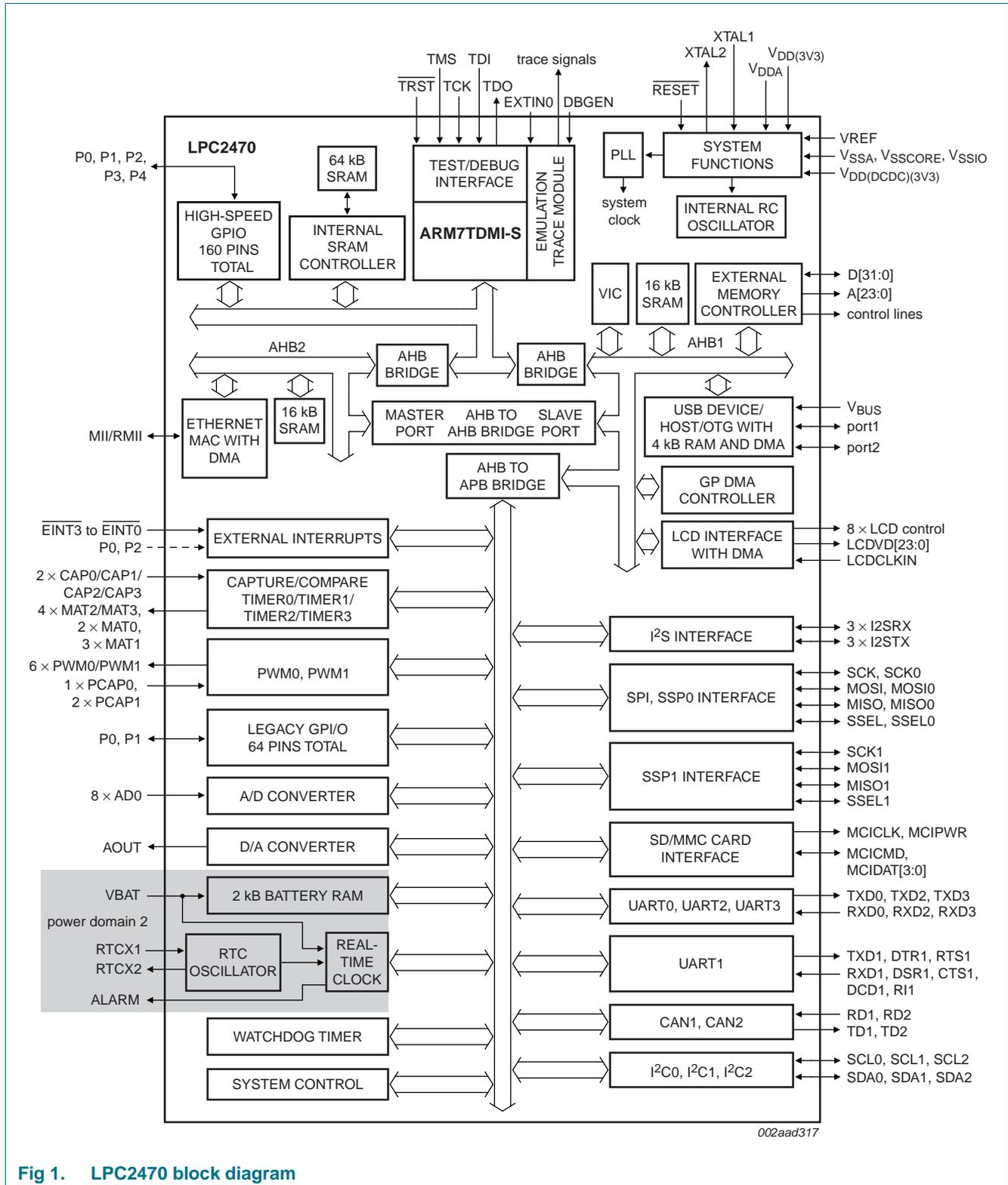
Fig 1. LPC2470 block diagram
