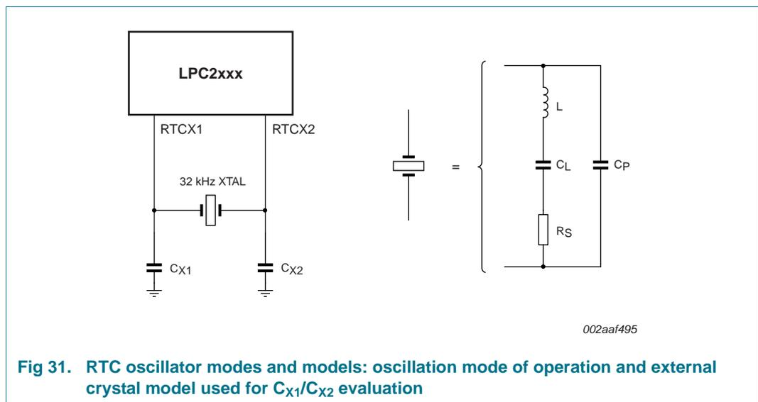
**Fig 31. RTC oscillator modes and models: oscillation mode of operation and external crystal model used for  $C_{X1}/C_{X2}$  evaluation**
