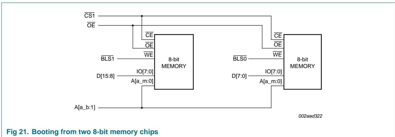
Fig 21. Booting from two 8-bit memory chips
