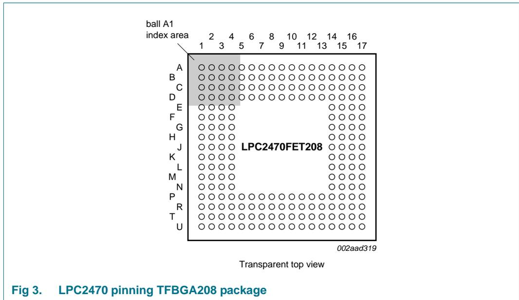
Fig 3. LPC2470 pinning TFBGA208 package
