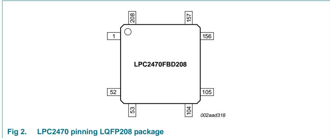
Fig 2. LPC2470 pinning LQFP208 package
