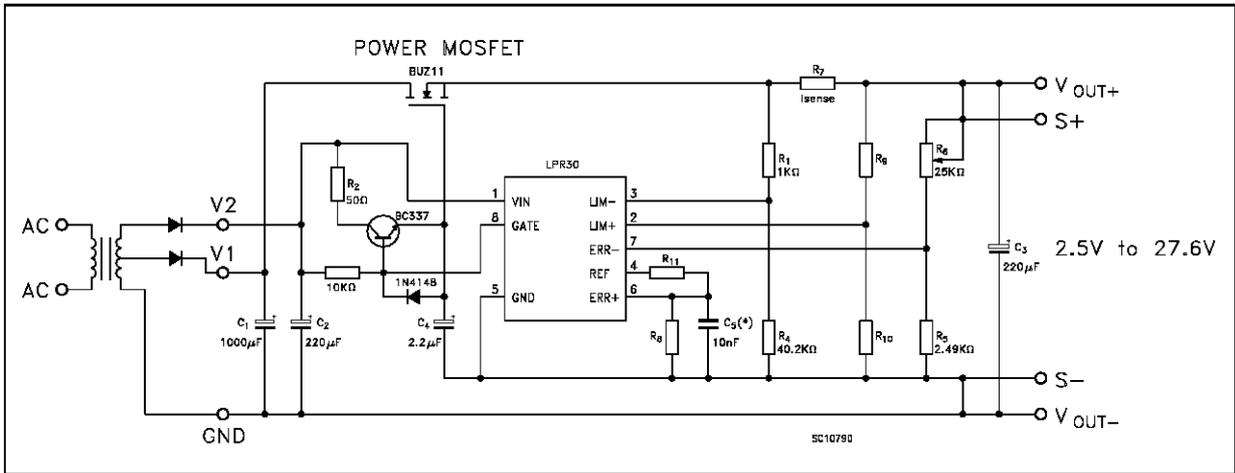
(\*) This capacitor improves noise performance; can be omitted in most applications
