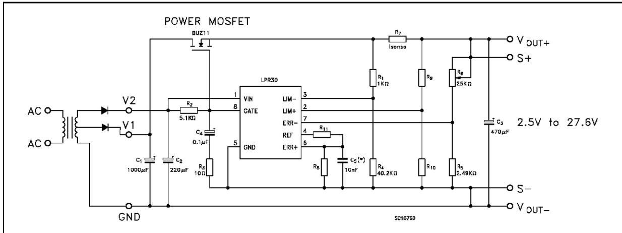
Figure 2: Configuration For Faster Response
