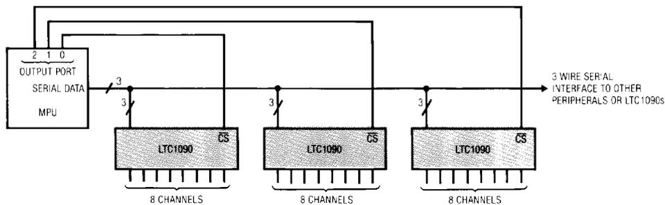
Figure 5. Several LTC1090s Sharing One 3 Wire Serial Interface
