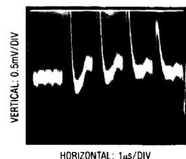
Figure 16. Poor Reference Settling Can Cause A/D Errors
