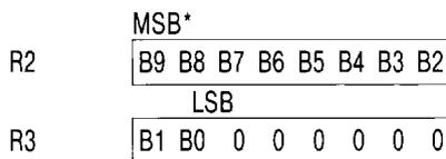
\*B9 is MSB in unipolar or sign bit in bipolar
