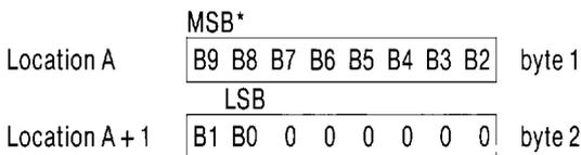
\*B9 is MSB in unipolar or sign bit in bipolar
