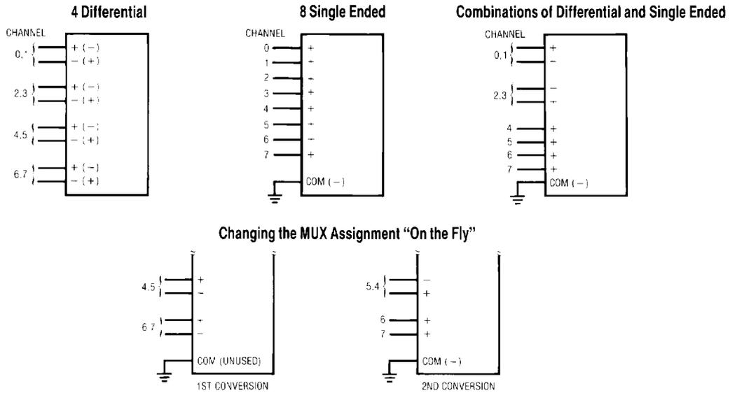
Figure 1. Examples of Multiplexer Options on the LTC1090
