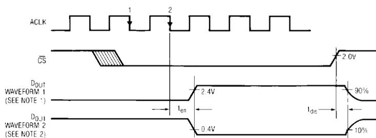
NOTE 1: WAVEFORM 1 IS FOR AN OUTPUT WITH INTERNAL CONDITIONS SUCH THAT THE OUTPUT IS HIGH UNLESS DISABLED BY THE OUTPUT CONTROL.
