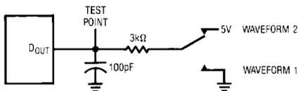
Load Circuit for  $t_{DDO}$ ,  $t_r$ , and  $t_f$
