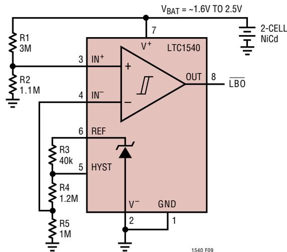
Figure 9. Low-Battery Detect Works Down to  $1.6\text{V}$
