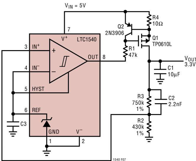
Figure 7. 3.3V Output Low Dropout Linear Regulator
