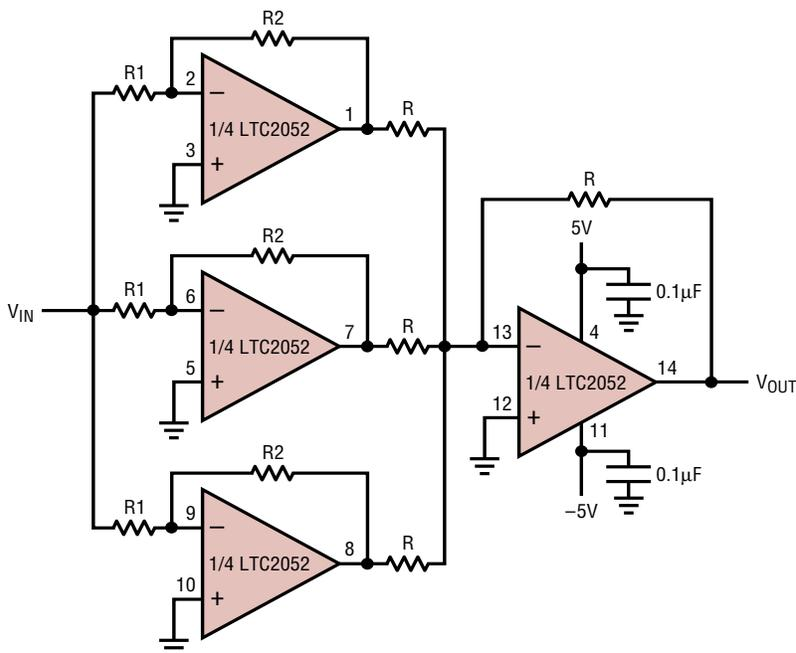
$$\frac{V_{OUT}}{V_{IN}} = 3 \frac{R_2}{R_1}; \text{ INPUT DC - 10Hz NOISE} \cong 0.8\mu\text{V}_{p-p} = \frac{\text{NOISE OF EACH PARALLEL OP AMP}}{\sqrt{3}}$$
