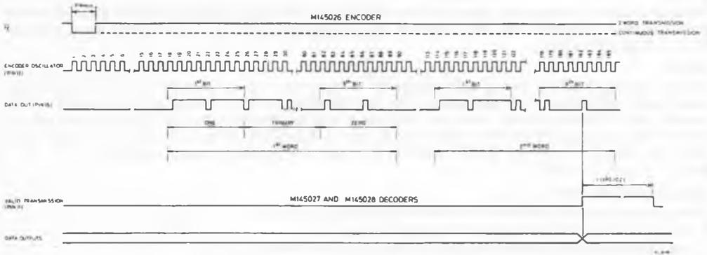
Figure 6 - Encoder Data Waveforms (M145026)
