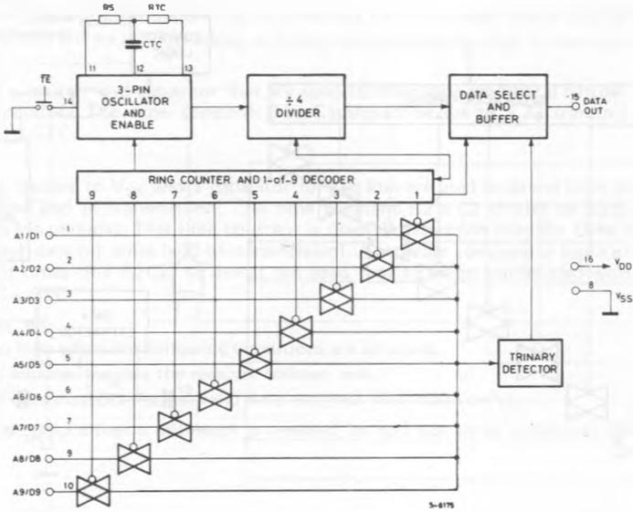
Fig. 2 - Decoder block diagram M145027
