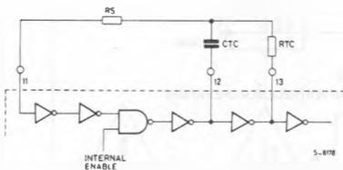
The value for  $RS$  should be chosen to be about 2 times  $RTC$ . This range will ensure that current through  $RS$  is insignificant compared to current through  $RTC$ . The upper limit for  $RS$  must ensure that  $RS \times 5 \text{ pF}$  (input capacitance) is small compared to  $RTC \times \text{CTC}$ .
