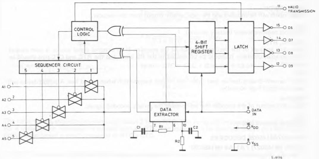
Fig. 3 - Decoder block diagram M145028
