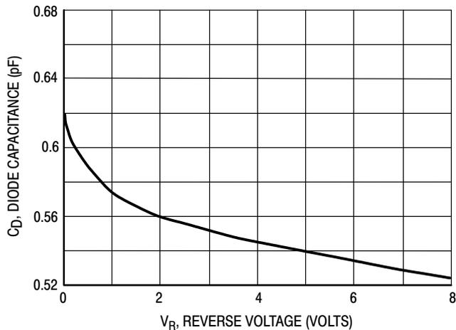
Figure 4. Diode Capacitance
