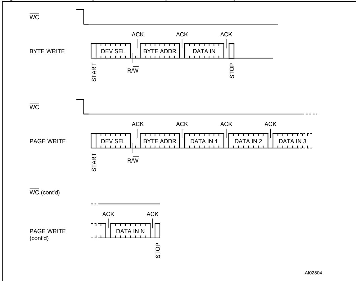
memory replies with an Ack. The master terminates the transfer by generating a STOP condition.
