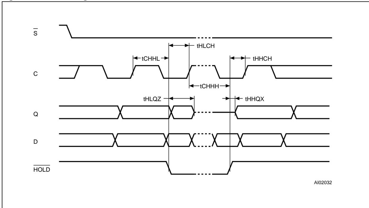
Figure 24. Output Timing
