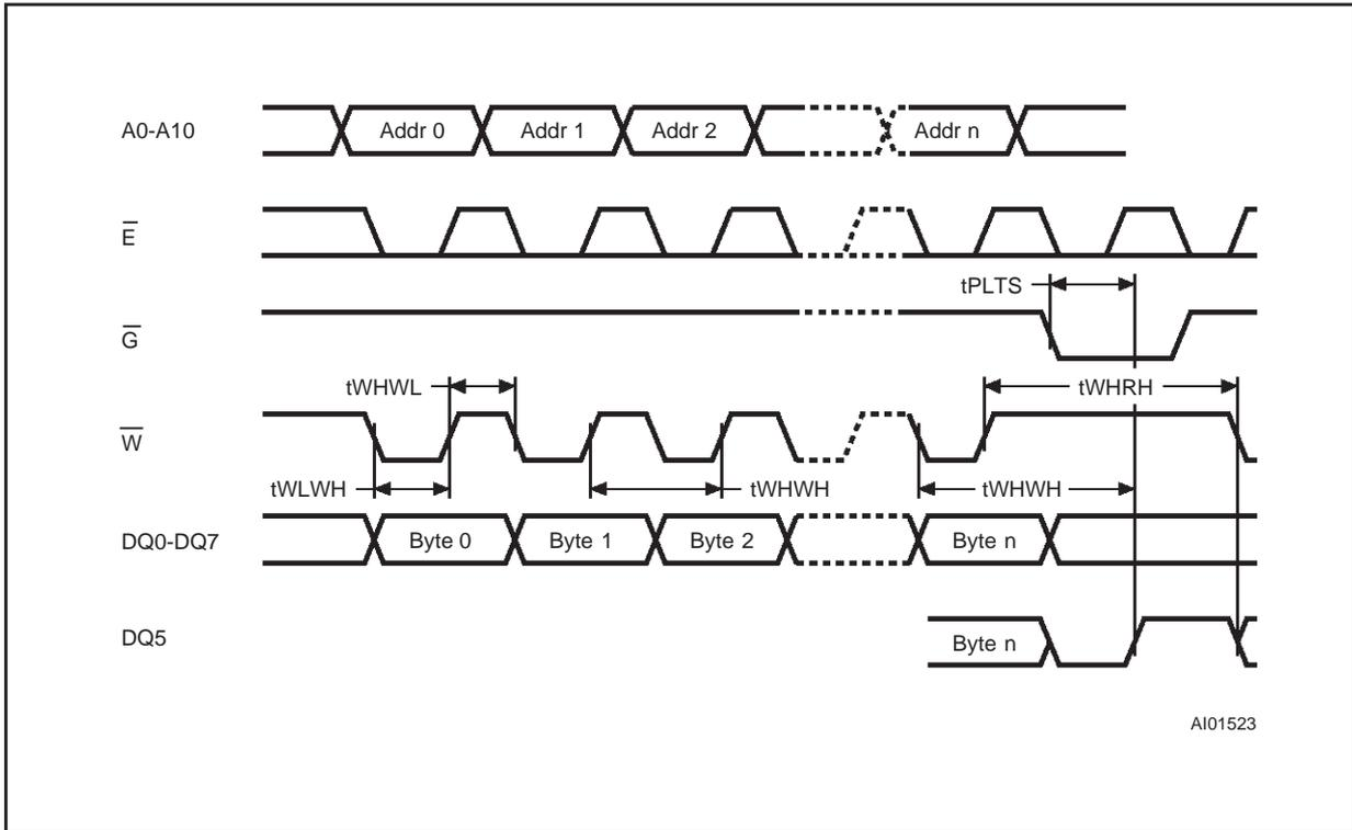
Figure 13. Software Protected Write Cycle Waveforms
