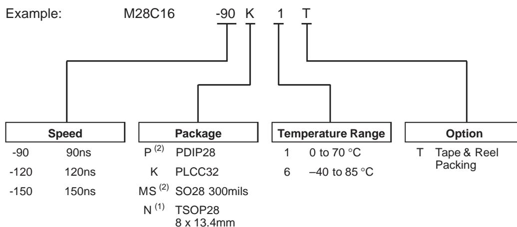
**Notes:** 1. The M28C16 in TSOP28 package has a Ready/Busy output on pin 1.
