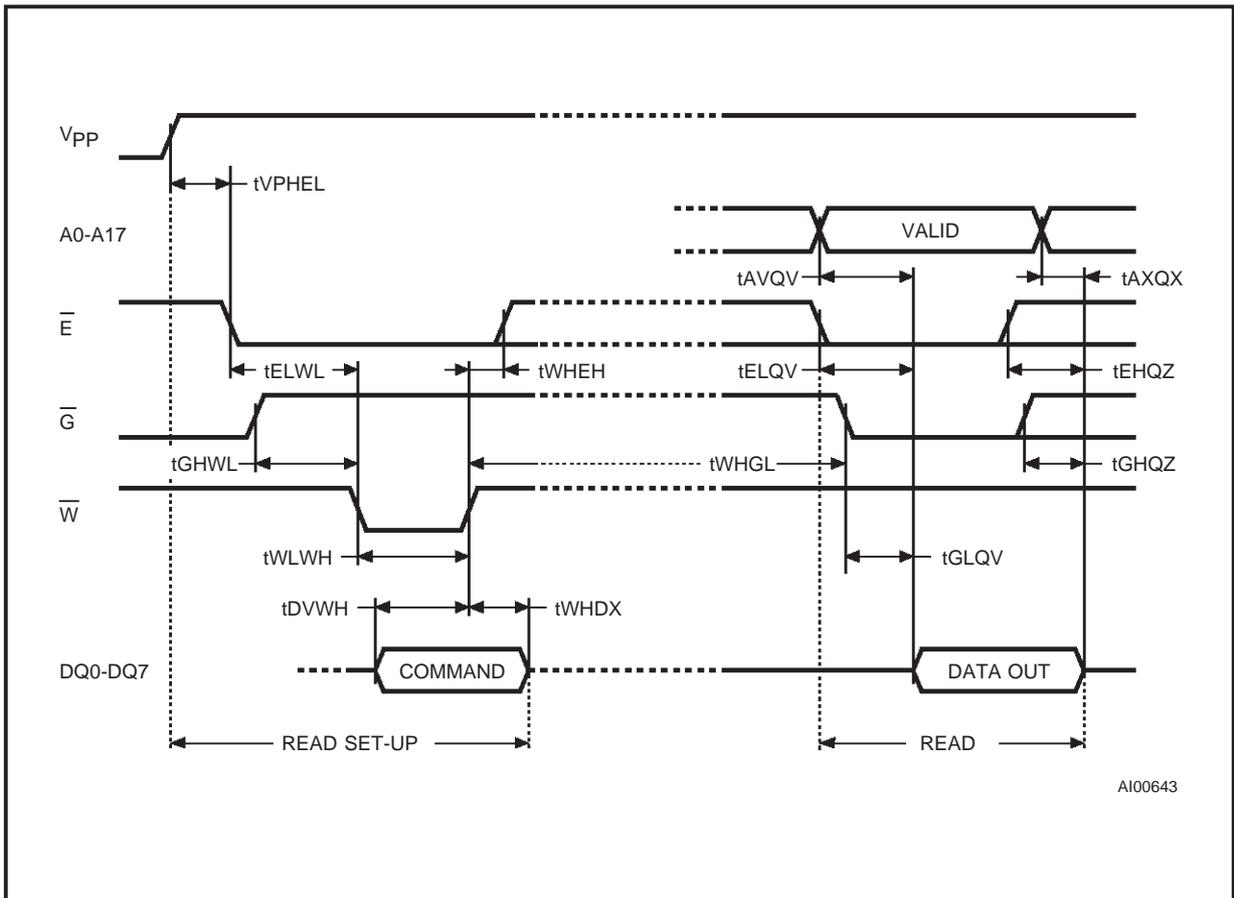
Figure 7. Electronic Signature Command Waveforms
