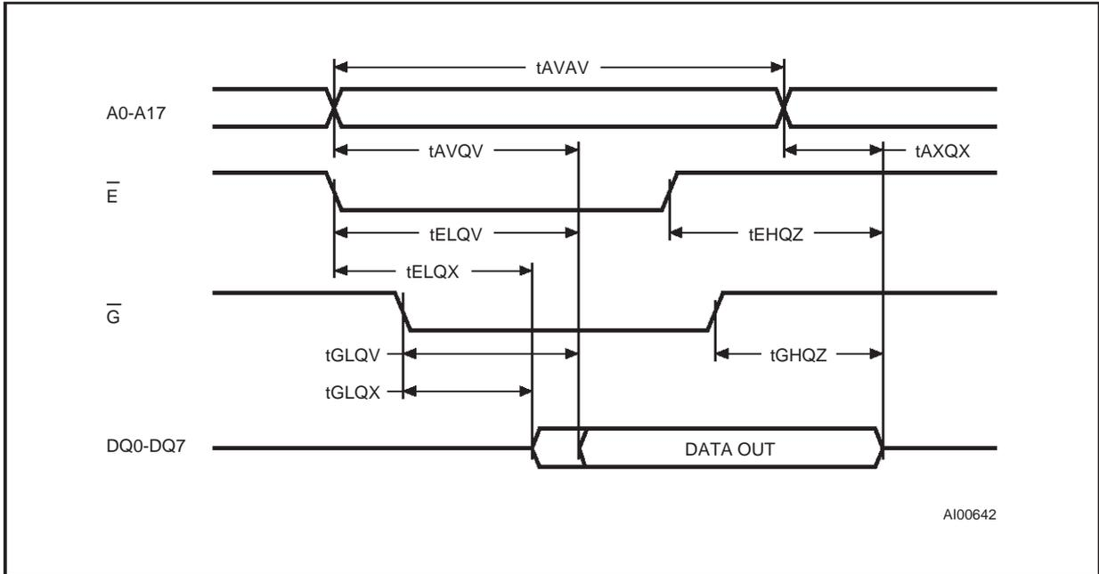
Figure 6. Read Command Waveforms
