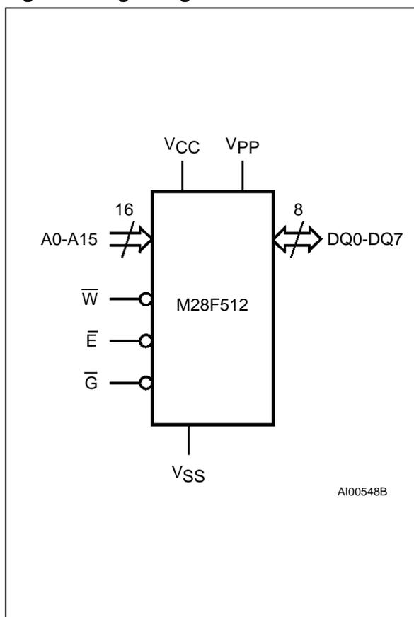
Figure 2A. DIP Pin Connections
