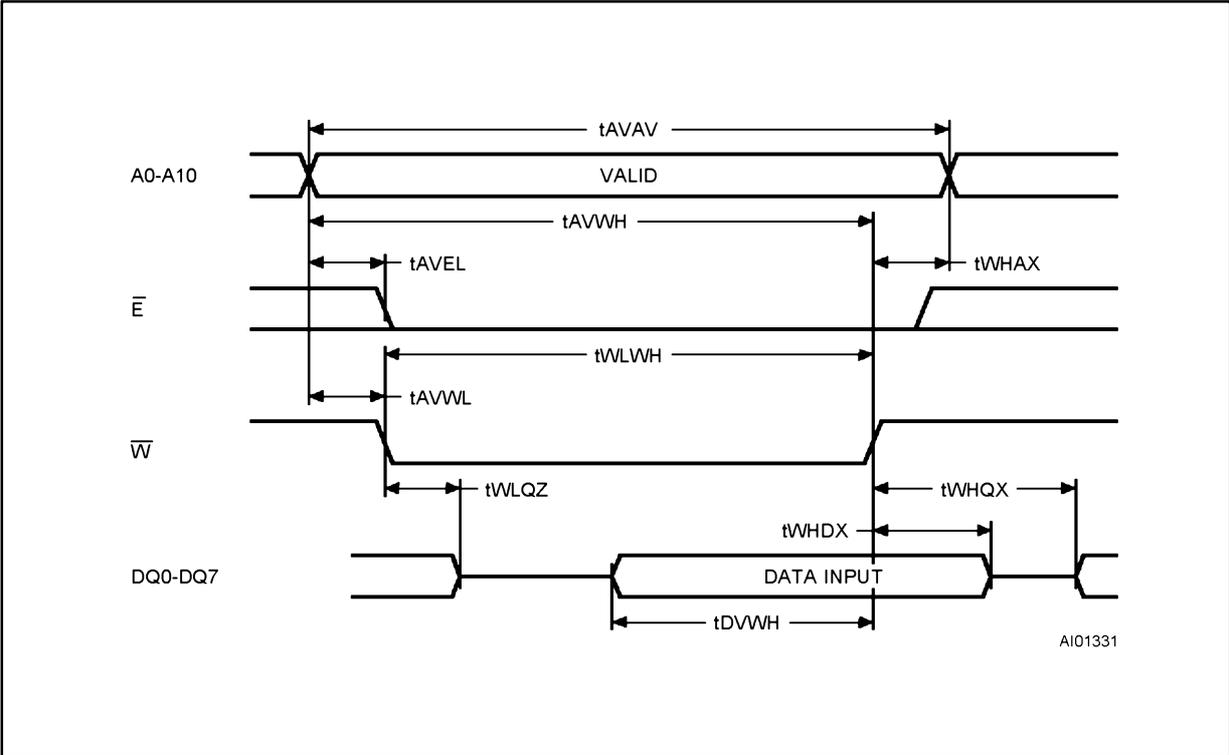
Figure 8. Chip Enable Controlled, Write AC Waveforms
