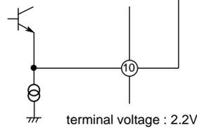
In the 4.5MHz application, the internal voltage gain is increased by 6-dB in comparison with the other applications and then the signals are delivered through an emitter follower.
