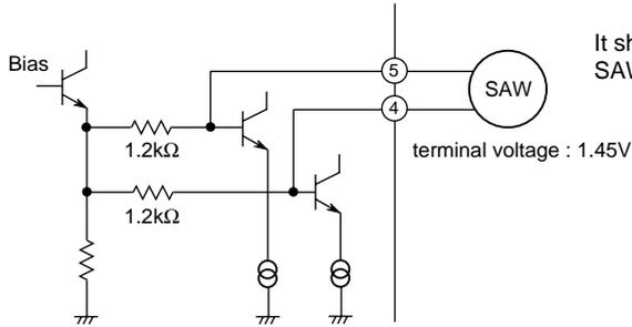
It should be designed considering careful impedance matching with the SAW filter.
