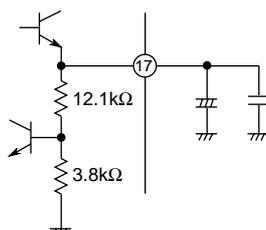
It is a regulated 5V output which has current drive capability of approximately 15 mA.
