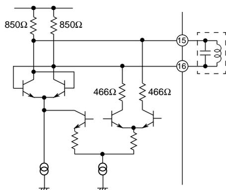
Connecting a tuning coil and capacitor to these pins enables an oscillation.
