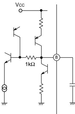
In spite of the 1-pin filter configuration, 2-pin filter characteristics are available by utilizing the dynamic AGC circuit.
