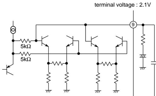
The FM detector can respond to several kinds of SIF signals without an adjustment and external components by adopting the PLL technique. It also is in compliance with the multi-SIF by selecting an appropriate deemphasis and audio output amplifier using the pin12 switch. The capacitor between pin 9 and 10, which fixes the deemphasis characteristics, can be determined considering the combination of an equivalent resistance of the IC and this capacitor itself.
