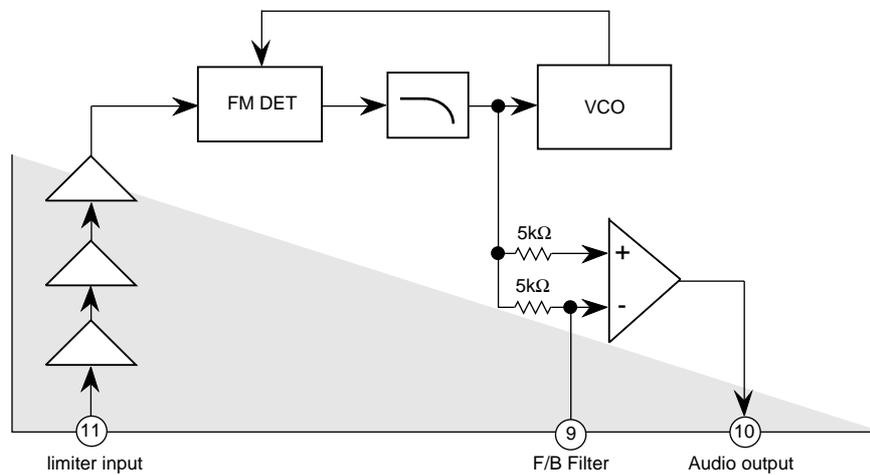
The input intercarrier signal from pin 11 is applied to the FM detector after amplifying in the limiting amplifiers.
