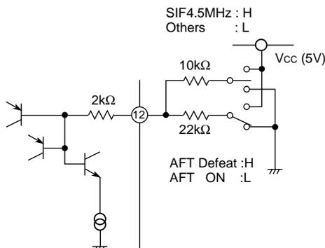
It works as a switch by connecting the resistor to 5V(High) of GND(Low), alternately.
