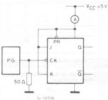
INPUT TRANSITION TIME IS THE SAME AS THAT IN CASE OF SWITCHING CHARACTERISTICS TEST
