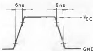
THE OTHER INPUTS ARE CONNECTED TO V<sub>CC</sub> LINE OR GND LINE.
