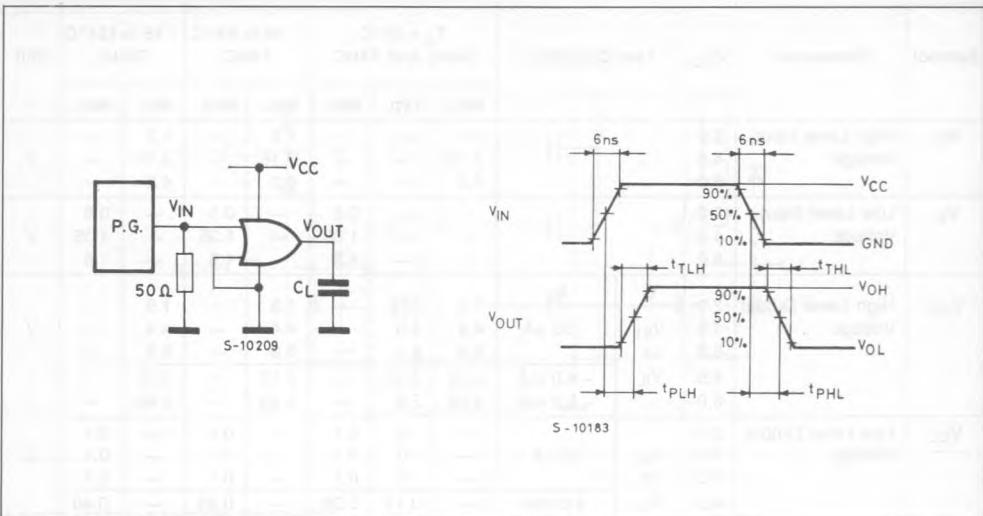
TEST CIRCUIT  $I_{CC}$  (Opr.)
