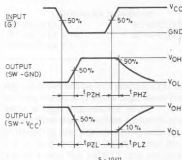
NOTE: SUCH A LOGIC LEVEL SHALL BE APPLIED TO EACH INPUT THAT THE OUTPUT VOLTAGE STAYS IN THE APPPOSITE SIDE TO THE SWITCH CONNECTION LEVEL, WHEN THE OUTPUT IS ENABLE
