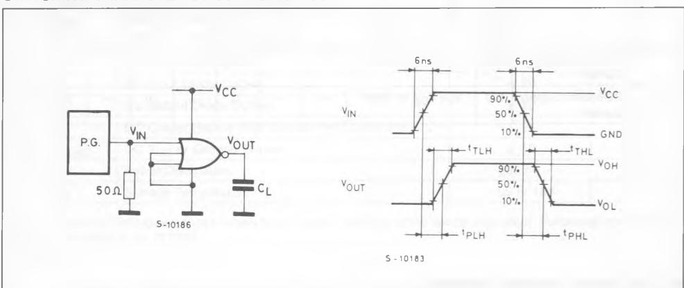
TEST CIRCUIT  $I_{CC}$  (Opr.)
