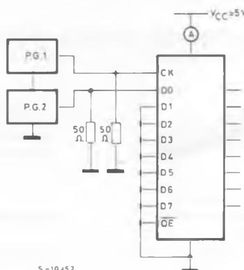
INPUT WAVEFORM IS THE SAME AS THAT IN CASE OF SWITCHING CHARACTERISTICS TEST.
