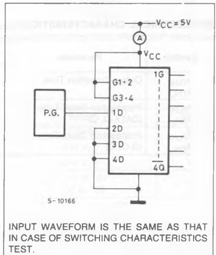
INPUT WAVEFORM IS THE SAME AS THAT IN CASE OF SWITCHING CHARACTERISTICS TEST.
