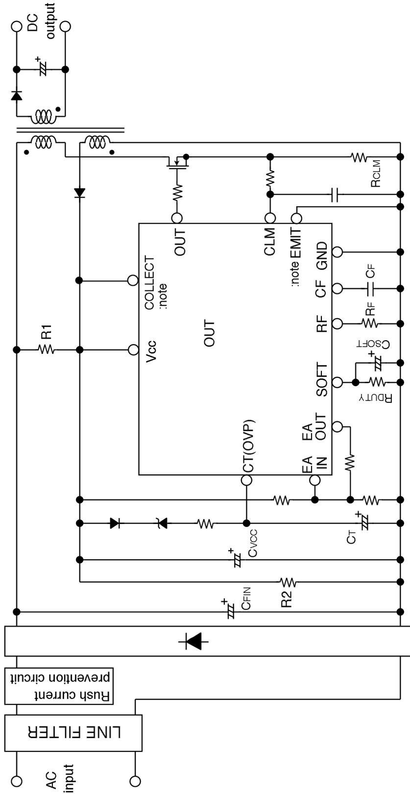
:note GND terminal is connected to emitter terminal as M62213FP in IC inside.
