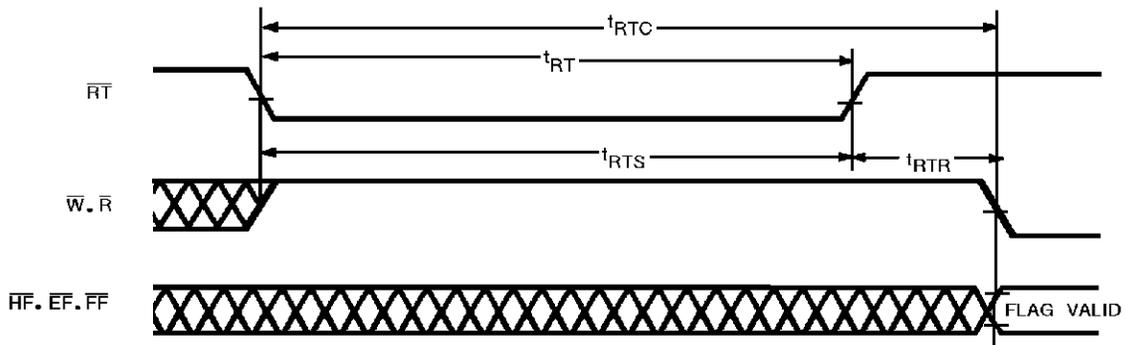
Note : 23.  $\bar{EF}$ ,  $\bar{FF}$  and  $\bar{HF}$  may change status during Retransmit, but flags will be valid at  $t_{RTC}$ .
