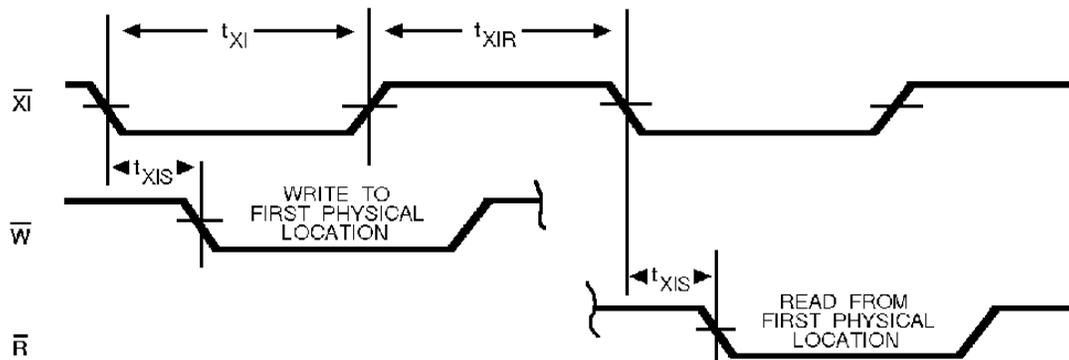
Figure 17. Read Data Flow – Through Mode.
