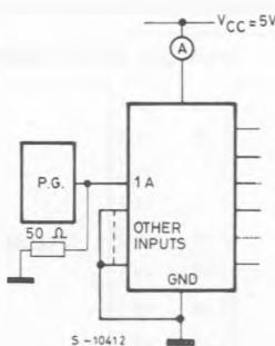
INPUT WAVEFORM IS THE SAME AS THAT IN CASE OF SWITCHING CHARACTERISTICS TEST
