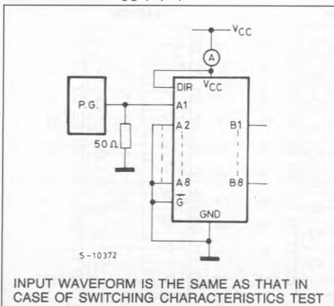
INPUT WAVEFORM IS THE SAME AS THAT IN CASE OF SWITCHING CHARACTERISTICS TEST
