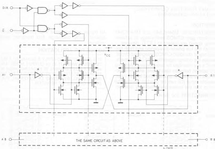
NOTE: IN CASE OF HC245 OR HC643, INPUT INVERTERS MARKED\* AT A BUS AND B BUS OR AT B BUS ARE ELIMINATED RESPECTIVELY
