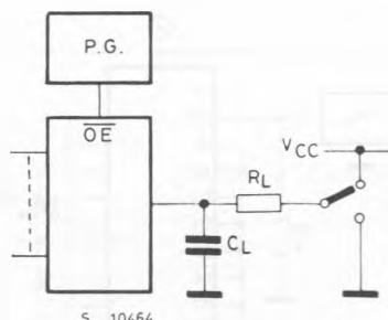
NOTE: EACH FLIP-FLOP WILL BE SET HIGH WHEN SWITCH IS CONNECTED TO GND LINE AND IT WILL BE SET LOW WHEN SWITCH IS CONNECTED TO VCC LINE.
