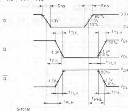
$t_{PLH}, t_{PHL} (LE - Q, \bar{Q})$
