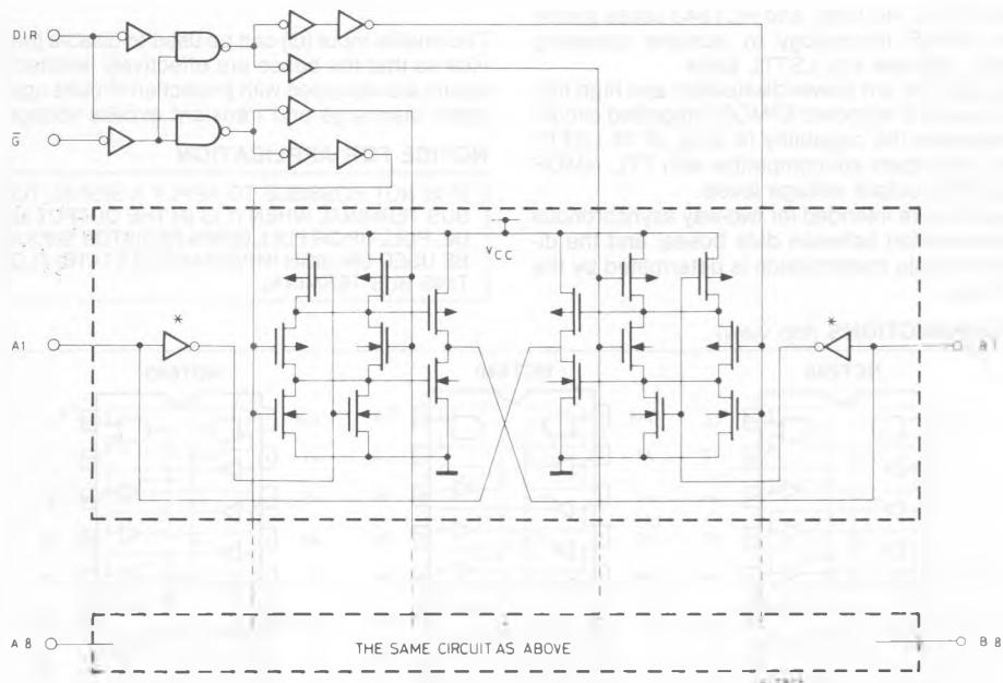
NOTE: IN CASE OF HCT245 OR HCT643, INPUT INVERTERS MARKED \* AT A BUS OR AT B BUS ARE ELIMINATED RESPECTIVELY.
