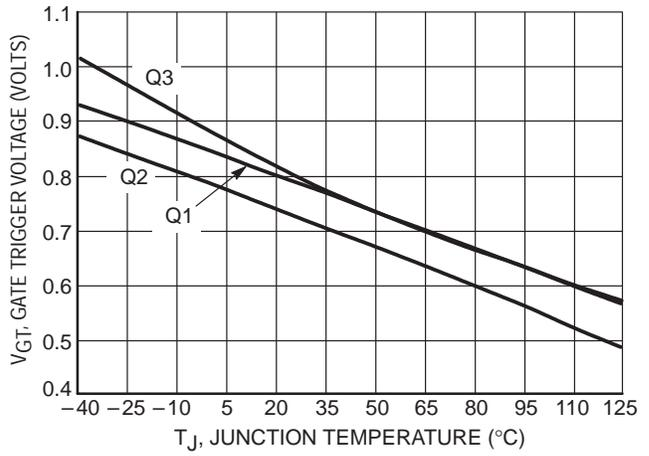
**Figure 2. Typical Gate Trigger Voltage versus Junction Temperature**
