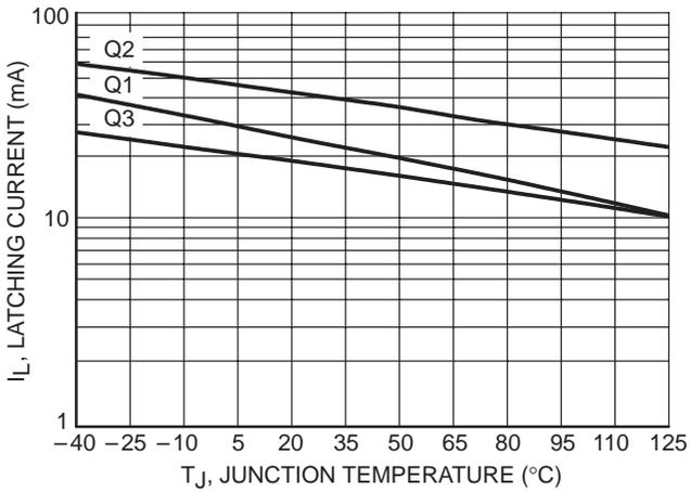
**Figure 3. Typical Latching Current versus Junction Temperature**
