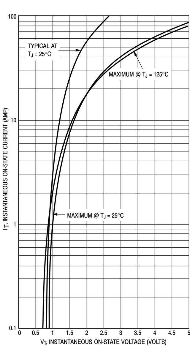
Figure 3. On-State Characteristics
