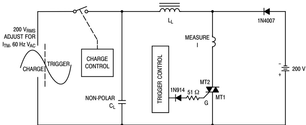
Note: Component values are for verification of rated (di/dt)<sub>c</sub>. See AN1048 for additional information.
