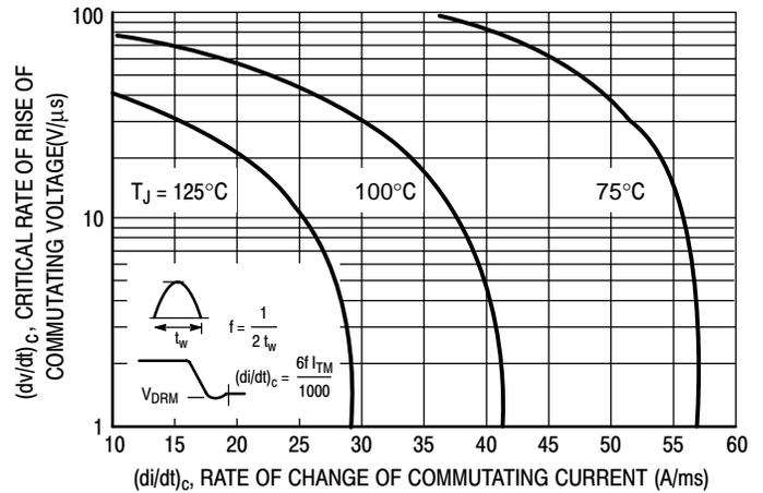
Figure 9. Critical Rate of Rise of Commutating Voltage
