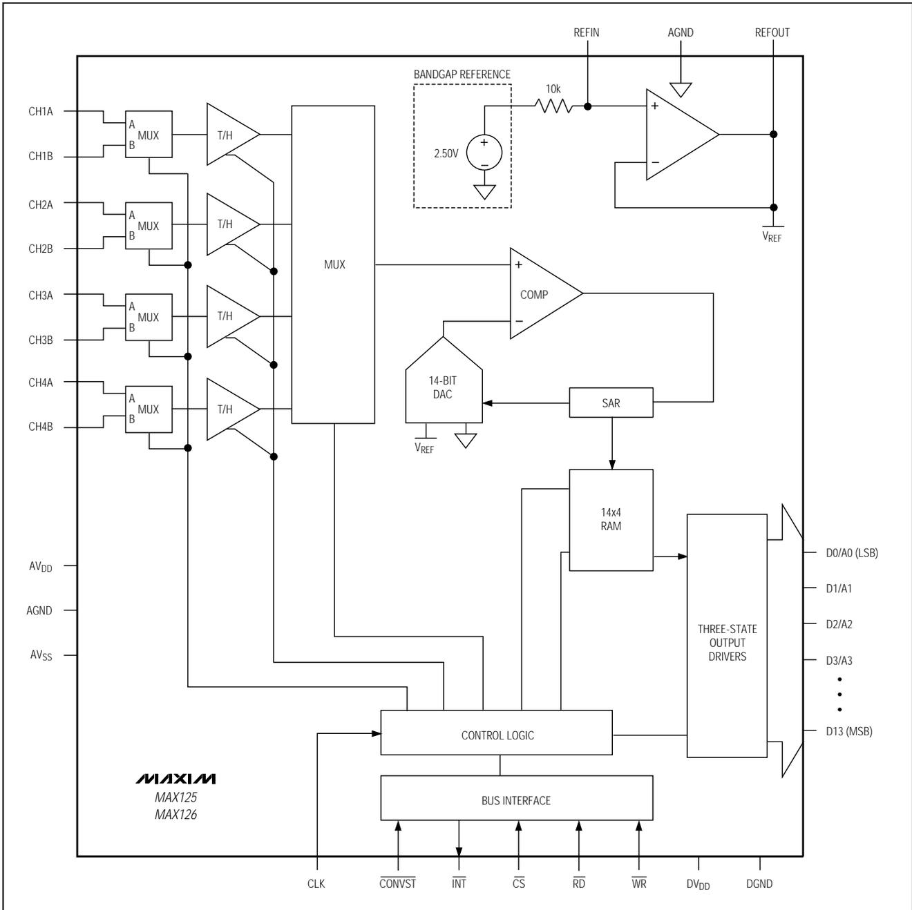
Figure 2. Functional Diagram
