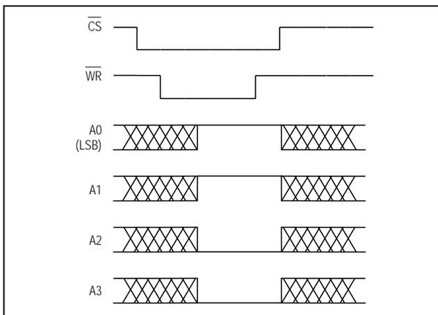
Figure 5. Programming a Four-Channel Conversion, Input Mux A
