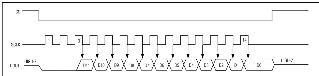
Figure 13. QSPI Serial Interface Timing (CPOL = 0, CPHA = 1)
