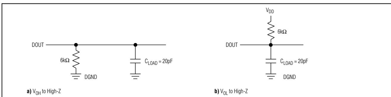
Figure 2. Load Circuits for DOUT Disable Time
