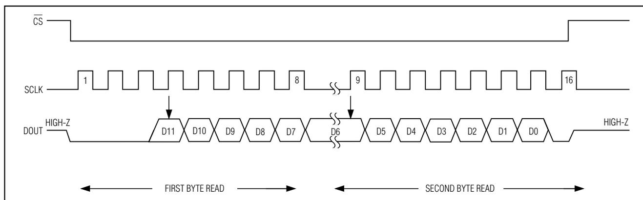
Figure 12. SPI/MICROWIRE Serial Interface Timing (CPOL = CPHA = 0)
