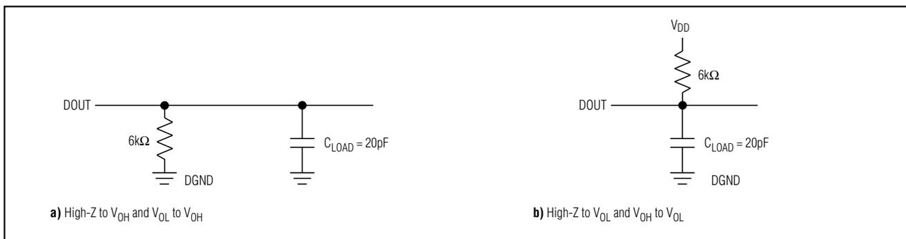
Figure 1. Load Circuits for DOUT Enable Time
