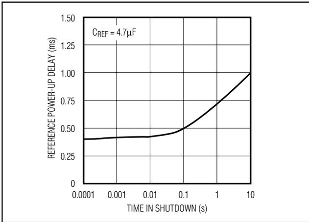
Figure 7. Reference Power-Up vs. Time in Shutdown
