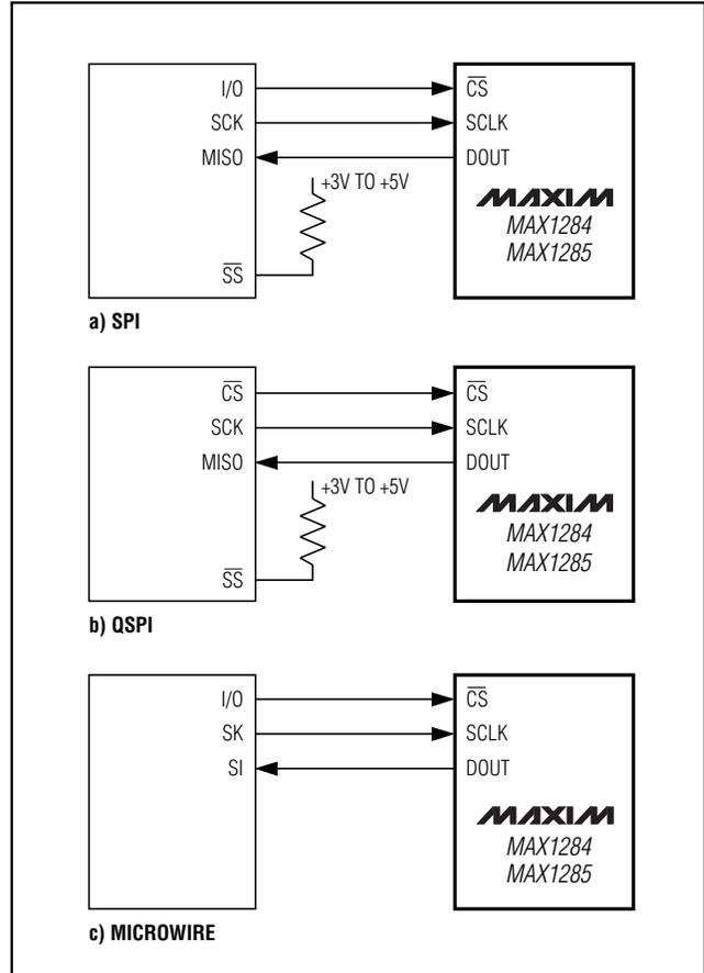
Figure 11. Common Serial-Interface Connections to the MAX1284/MAX1285
