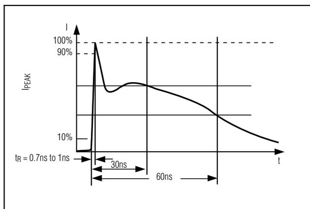
Figure 3. IEC 61000-4-2 ESD Generator Current Waveform
