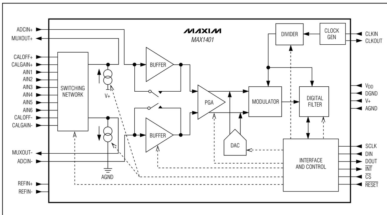
Figure 2. Functional Diagram
