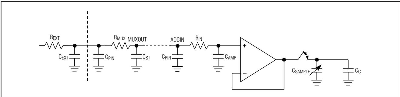
Figure 6. Analog Input, Buffered Mode (BUFF = 1)
