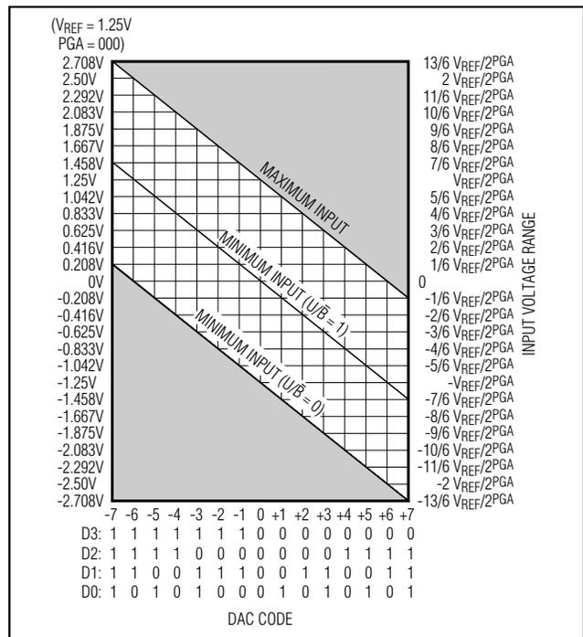
Figure 9. Input Voltage Range vs. DAC Code
