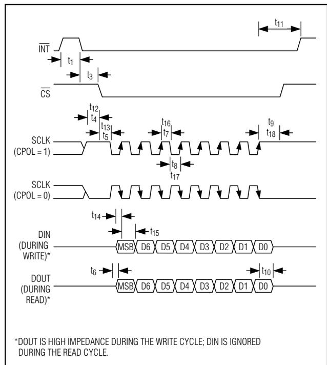
Figure 4. Serial-Interface Timing
