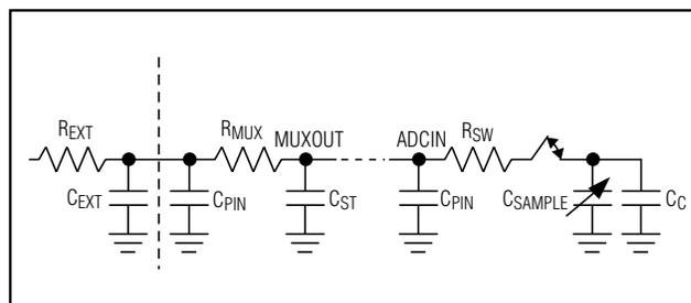
Figure 5. Analog Input, Unbuffered Mode (BUFF = 0)
