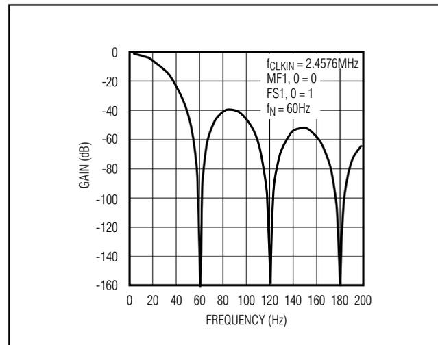
Figure 10. Frequency Response of the SINC<sup>3</sup> Filter (Notch at 60Hz)
