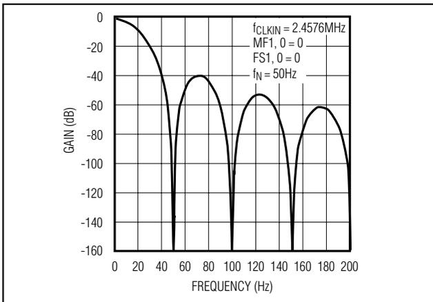
Figure 11. Frequency Response of the SINC<sup>3</sup> Filter (Notch at 50Hz)
