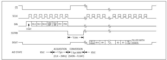
Figure 9. Internal Clock Mode Timing
