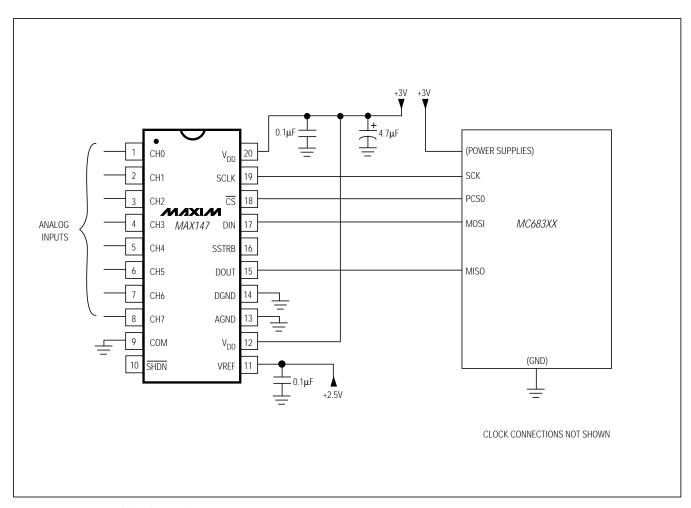
Figure 17. MAX147 QSPI Connections
