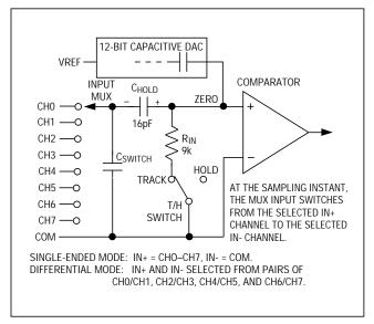
Figure 4. Equivalent Input Circuit
