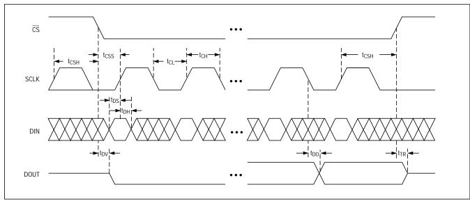
Figure 7. Detailed Serial-Interface Timing
