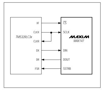
Figure 18. MAX147-to-TMS320 Serial Interface
