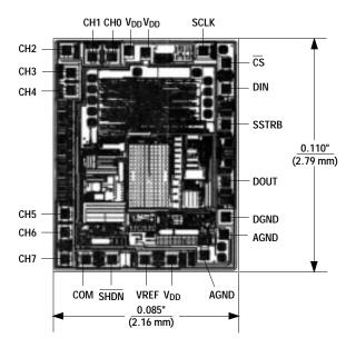
TRANSISTOR COUNT: 2554 SUBSTRATE CONNECTED TO DGND
