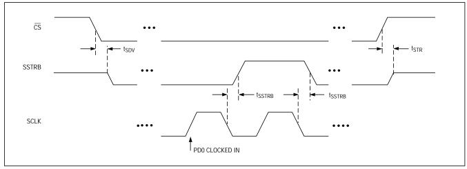
Figure 8. External-Clock-Mode SSTRB Detailed Timing
