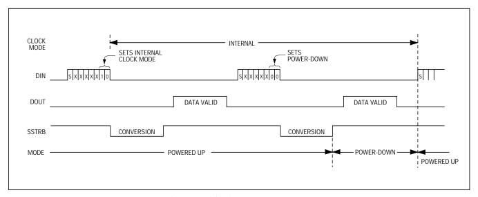
Figure 12b. Timing Diagram Power-Down Modes, Internal Clock
