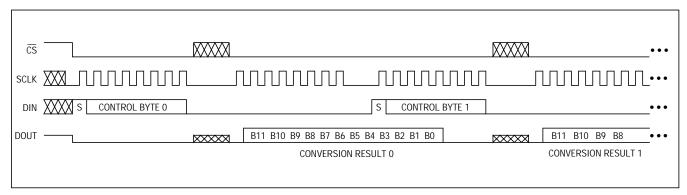
Figure 11b. External Clock Mode, 16 Clocks/Conversion Timing
