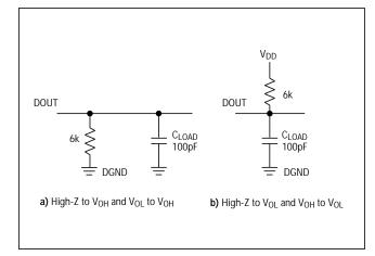
Figure 1. Load Circuits for Enable Time
