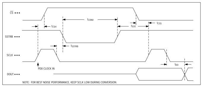
Figure 10. Internal Clock Mode SSTRB Detailed Timing
