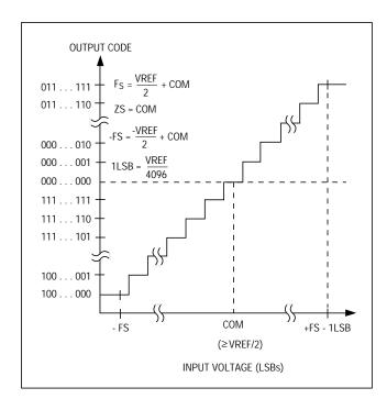
Figure 15. Bipolar Transfer Function, Full Scale (FS) = VREF/2 + COM, Zero Scale (ZS) = COM
