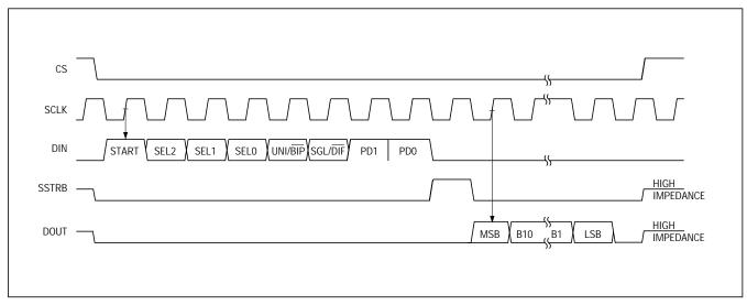
Figure 19. TMS320 Serial-Interface Timing Diagram
