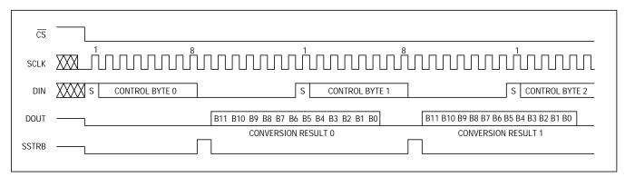
Figure 11a. External Clock Mode, 15 Clocks/Conversion Timing
