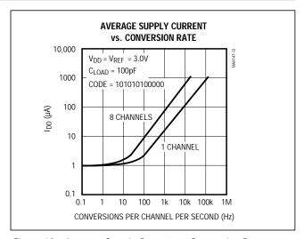
Figure 13. Average Supply Current vs. Conversion Rate
