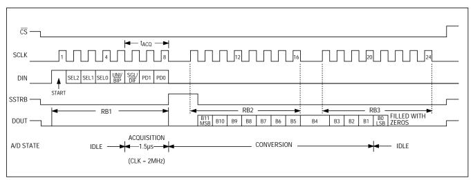
Figure 6. 24-Bit External-Clock-Mode Conversion Timing (Microwire and SPI Compatible, QSPI Compatible with fCLK ≤ 2MHz).
