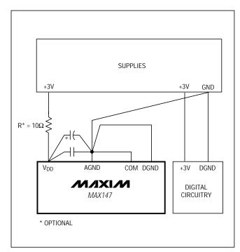
Figure 16. Power-Supply Grounding Connection
