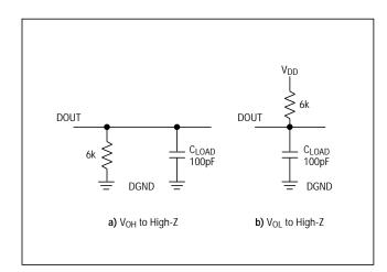
Figure 2. Load Circuits for Disable Time
