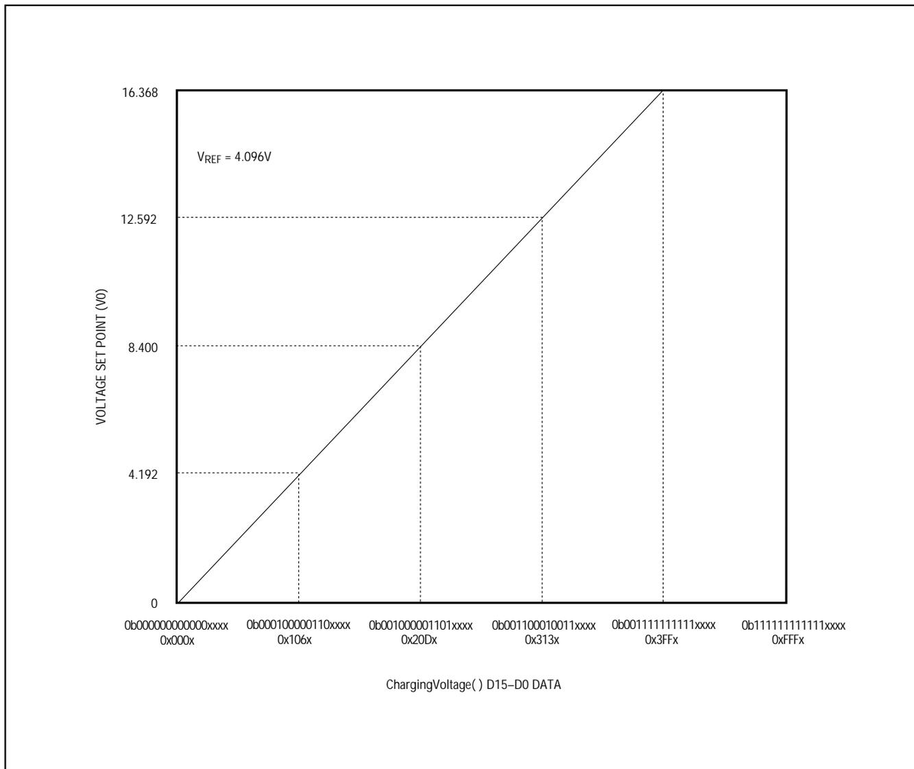
Figure 8. ChargingVoltage( ) Data to Voltage Mapping
