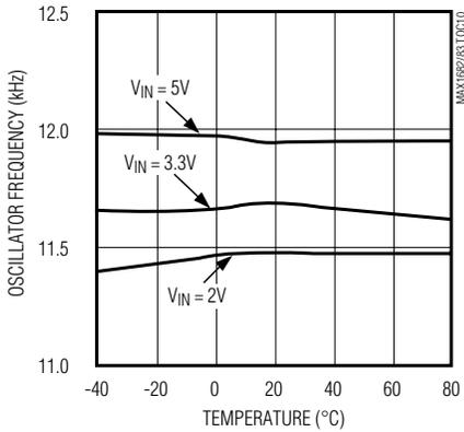
**MAX1683 OSCILLATOR FREQUENCY vs. TEMPERATURE**
