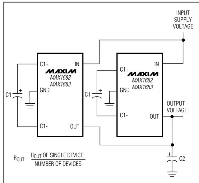
Figure 4. Paralleling Devices
