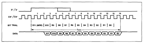
Figure 4. MAX171 Conversion Cycle Timing
