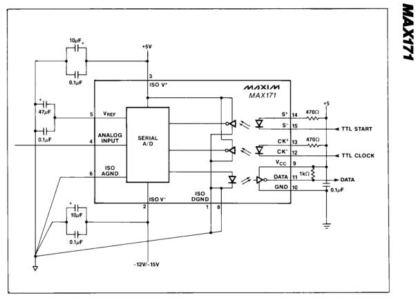
Figure 1. MAX171 Operating Circuit
