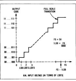
Figure 6. MAX171 Transfer Function
