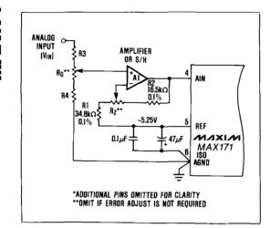
Figure 8. MAX171 Non-Inverting Bipolar Operation
