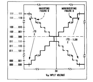
Figure 10. Ideal Input/Output Transfer Characteristics for the Bipolar Circuits in Figures 8 and 9
