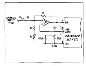
Figure 9. MAX171 Inverting Bipolar Operation
