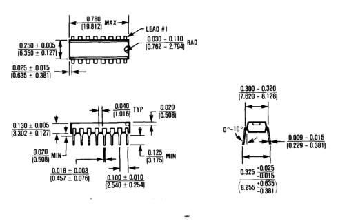
**16 Lead Plastic DIP (PE)**  $\theta_{JA} = 135^{\circ}C/W$  $\theta_{JC} = 65^{\circ}C/W$
