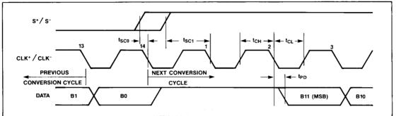
Figure 5. MAX171 Timing Diagram
