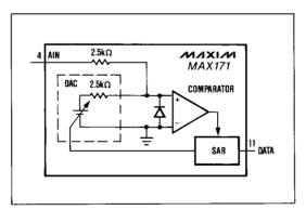
Figure 2. MAX171 Analog Equivalent Circuit
