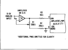
Figure 7. Full-Scale Adjustment
