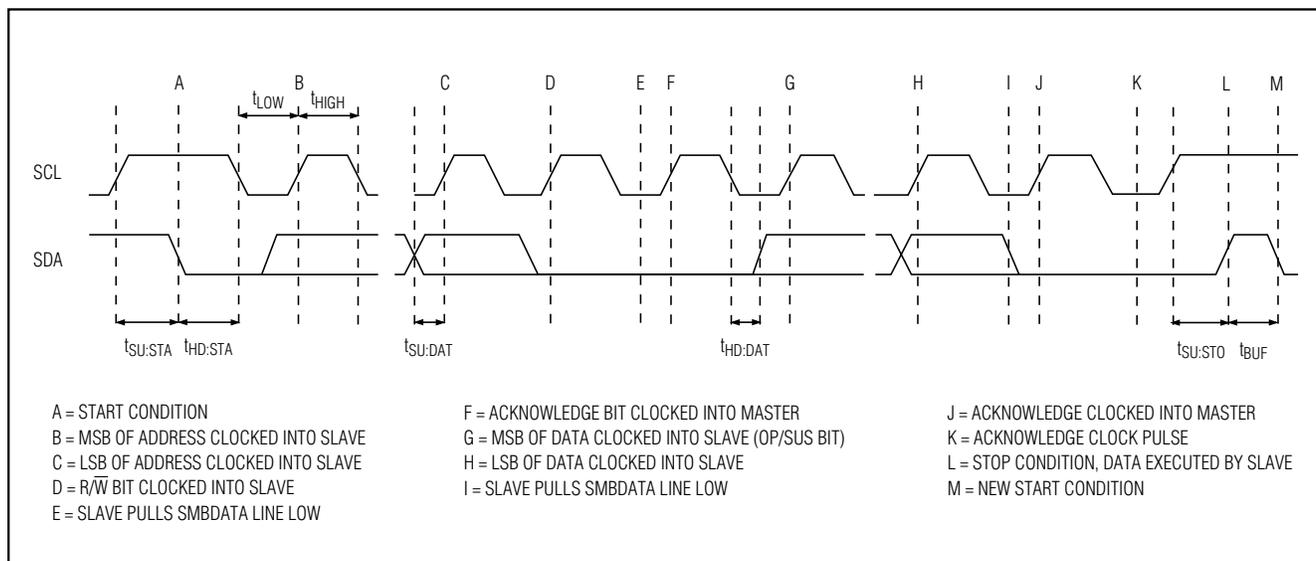
Figure 2. I<sup>2</sup>C-Compatible Serial-Interface Timing Diagram
