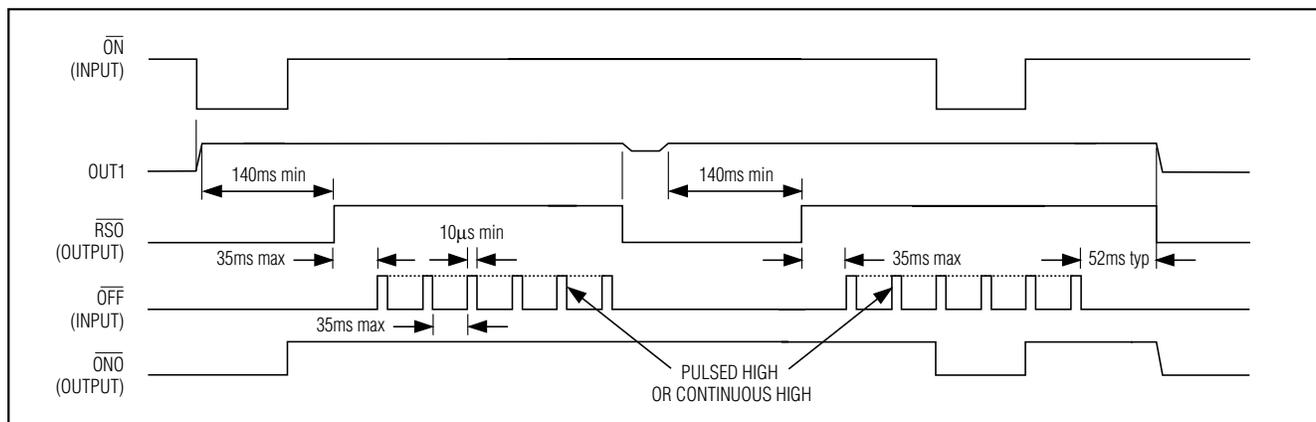
Figure 3. Push-On/Push-Off Startup and Shutdown Timing Diagram
