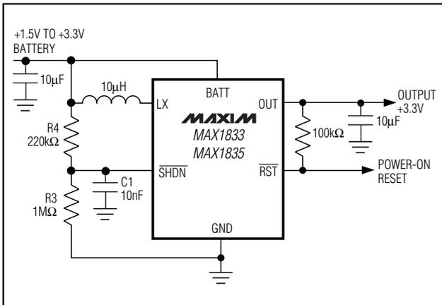
Figure 1a. MAX1833/MAX1835 Typical Operating Circuit
